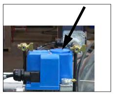
Figure 4-8 Main Gas Choke - High Fire Adjustment
