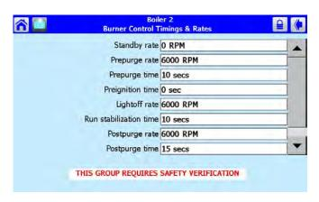
Fig. 43. Burner Control Timings and Rates configuration.
