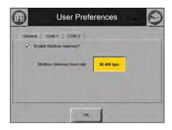
**NOTE:** The Modbus Gateway must be enabled at *each* boiler in the lead lag network (not just the Master host) for individual boiler status monitoring.
