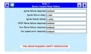
Fig. 45. Burner Control Flame Failure configuration.
