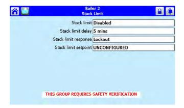
Fig. 37. Stack Limit configuration.
