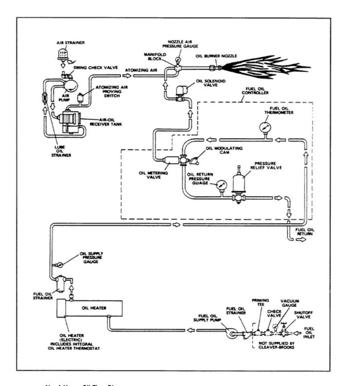
FIGURE 1-9. No. 4 Heavy Oil Flow Diagram
