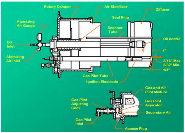
FIGURE 5-8. Burner Drawer with Gas Pilot
