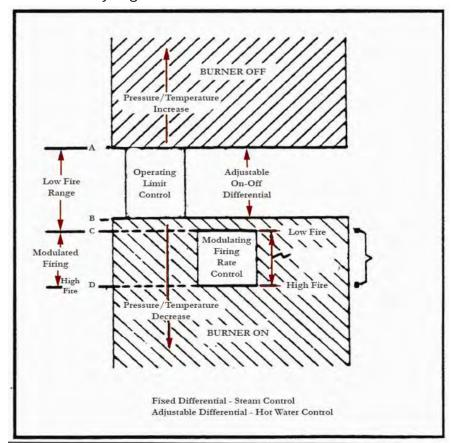
FIGURE 5-4. Operating Control and Modulating Actions
