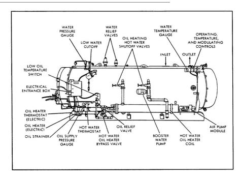
FIGURE 1-2. Typical Hot Water Boiler
