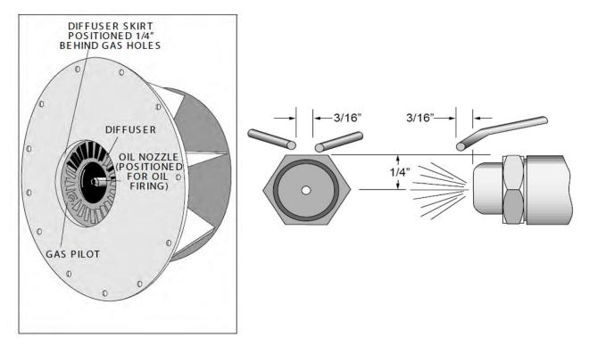
FIGURE 5-9. Diffuser and Oil Pilot Electrode
