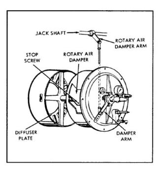
The stop screw in the rotary air damper limits damper travel at both closed (low fire) and fully opened (high fire) positions. This screw is provided so that it is possible to tell, even with the burner in place, whether the damper rotor is in fully opened or closed position by rotating the damper open and closed by means of the damper arm. Normally, the rate of flow of air through the damper with the rotor in low fire position is about one-third of maximum.
