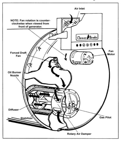
FIGURE 1-6. Secondary Air Flow
