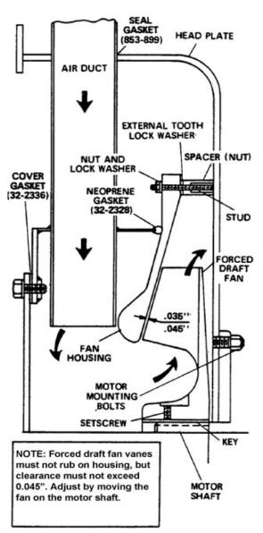
Check occasionally to see that the fan is securely tightened to the motor shaft. Check the clearance between the fan vanes and housing as outlined above. If the boiler is installed in a dusty location, check the vanes for deposits of dust or dirt since these buildups can cause a decrease in air capacity or lead to an unbalanced condition.
