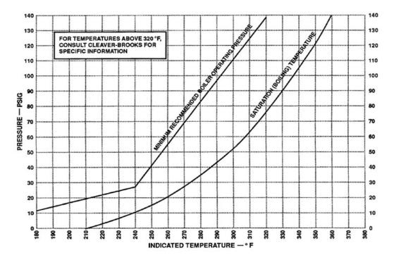
FIGURE 2-2. Pressure-Temperature Chart for Hot Water Boilers
