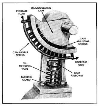
FIGURE 5-2. Modulating Cam
