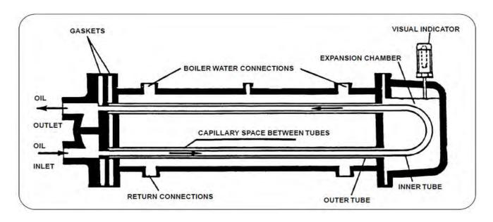
FIGURE 7-11. Circulation Layout of Hot Water Oil Heater (Alstrom)
