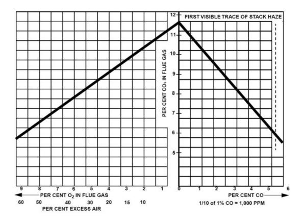
FIGURE 5-5. Flue Gas Analysis Chart for Natural Gas
