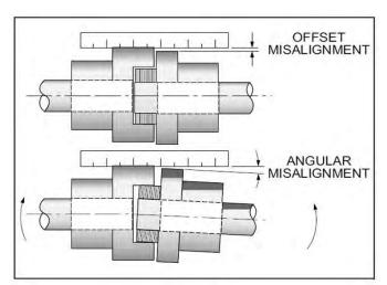
The coupling must be checked for both parallel (offset) alignment and angular (gap) alignment. Parallel misalignment exists when shaft axes are parallel but not concentric. Angular misalignment is the reverse situation, the shaft axes are concentric but not parallel.
