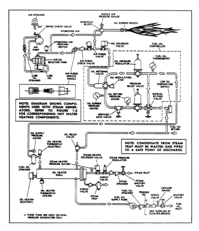
FIGURE 1-8. Heavy Oil Flow Diagram (Steam-Electric Heater
