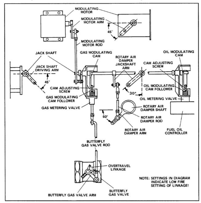
FIGURE 5-1. Complete Linkage Assembly: Combination Gas and Oil
