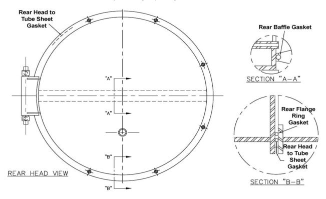
FIGURE 7-10. Rear Door Sealing
