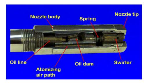
FIGURE 7-3. Burner Nozzle Assembly
