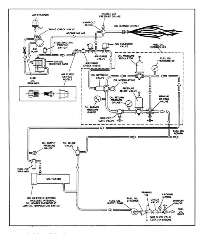
FIGURE 1-10. No. 5 Heavy Oil Flow Diagram
