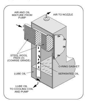
Pads of steel wool are used in this tank as a filtering medium to separate the lube oil from the compressed air.
