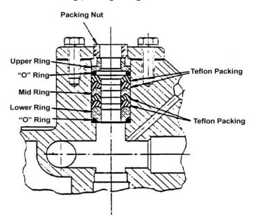
**8.**Lightly coat the stem with the lubricant provided with the packing kit. Place the new packing, o-rings, and guides onto the stem in the sequence shown in Figure 7-5. The beveled face of the guides and the Teflon rings must face upward, with the exception of the upper brass guide which is faced down. Make sure that the o-rings are properly located.
