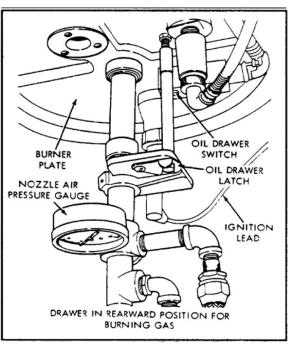
FIGURE 4-1. Positions of Burner Drawer for Oil and Gas
