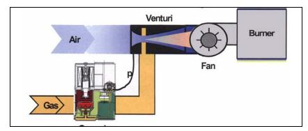
Figure 4-12 Premix Burner Technology - Full Modulation
