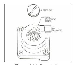
Figure 4-18 Regulating Adjusting Screw - Low Fire Offset
