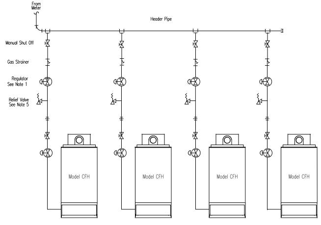
Figure 2-5 Typical gas header piping
