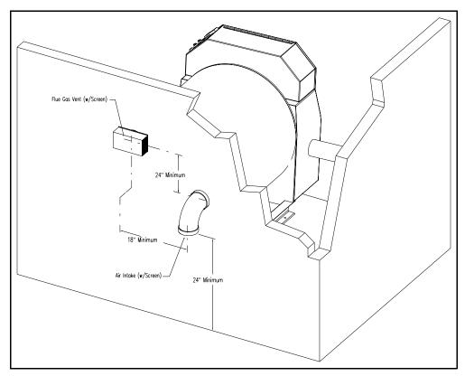
Figure 3-2 Horizontal Thru-wall Direct Venting System Category III Installation (Sealed Combustion Air/Stack Venting)
