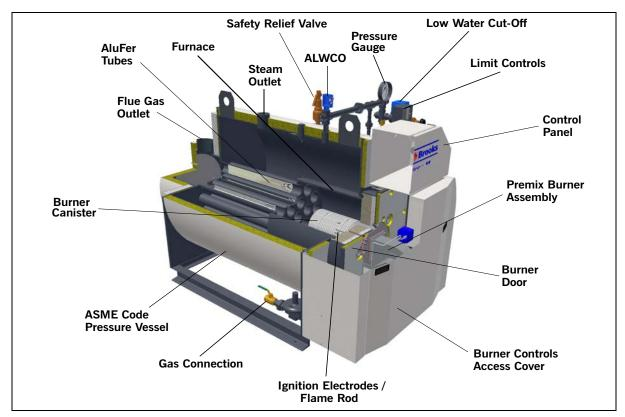
Figure 1-9 Model CFH Steam Boiler
