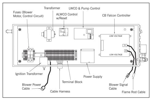
Figure 1-3 Model CFH Electrical Panel Interior
