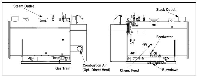
Figure 2-3 CFH Steam Boiler Connections
