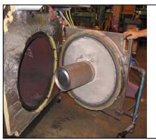
Figure 5-6 Burner assembly open
