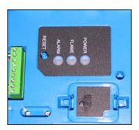
Figure 4-3 Controller status LEDs and reset button
