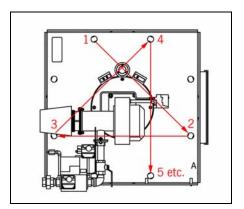
Figure 5-8 Fastening burner door
