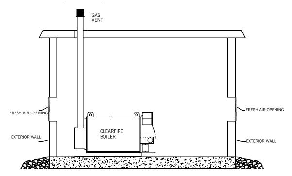
Figure 3-8. Engineered Method
