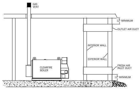
Figure 3-6. Two Opening Ducted Method
