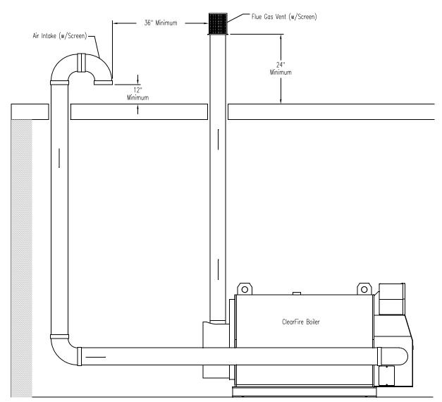
Figure 3-9. Direct Vent Combustion
