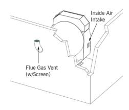
Figure 3-1 Horizontal Venting Thru-Wall Using Inside Air For Combustion
