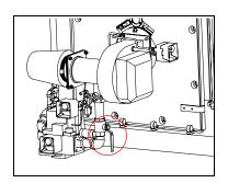
Figure 4-13 Manual Gas Shut-Off (downstream)
