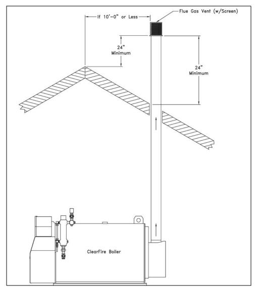
Figure 3-3 Vertical Stack with Inside Combustion Air
