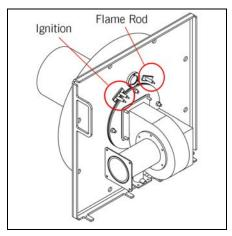
Figure 5-5 Electrode connections
