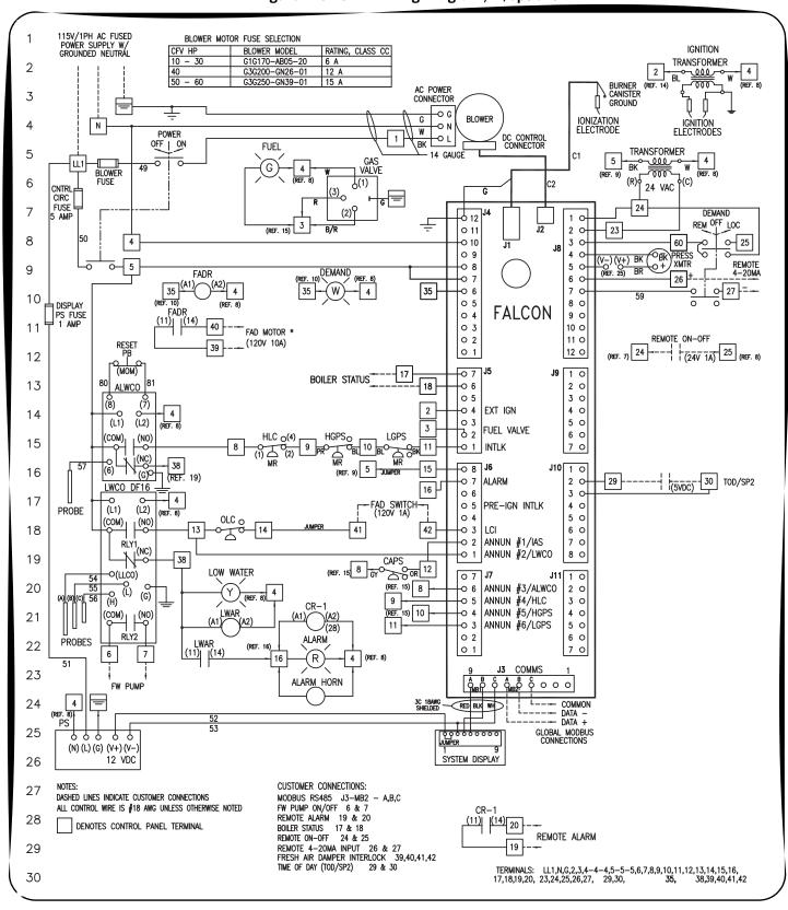
Figure 2-9 CFH Wiring Diagram, w/options
