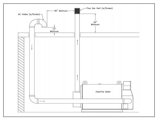
Figure 3-4 Vertical Stack with Direct Vent Combustion Air
