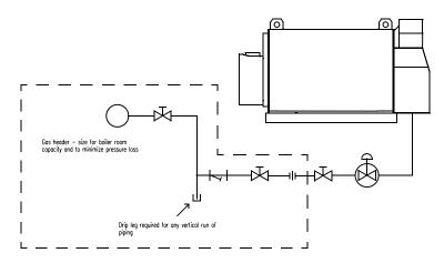
Figure 2-6 Example gas piping <1 psig supply
