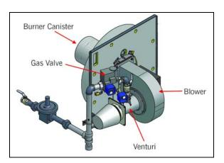
**Figure 1-5 Burner Components**
