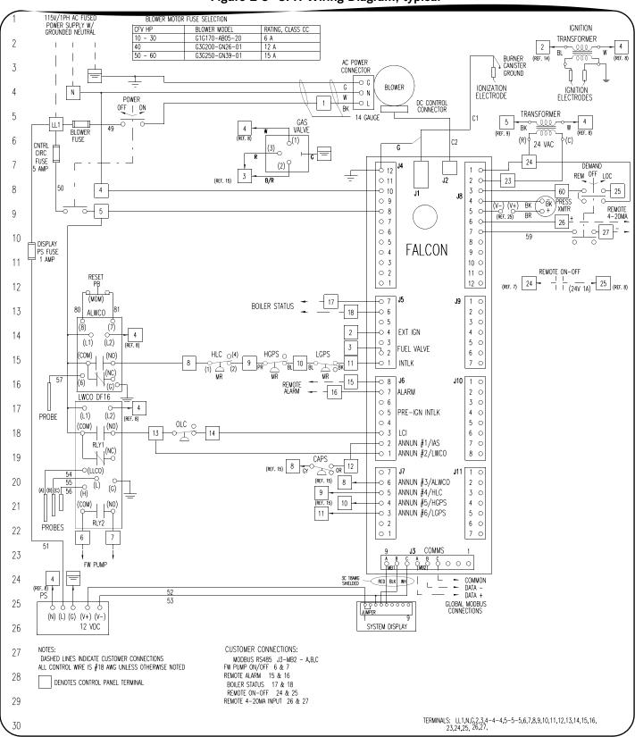
Figure 2-9 CFH Wiring Diagram, typical
