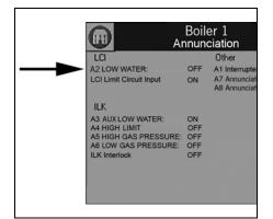
Figure 4-17 Low Water Cutoff test
