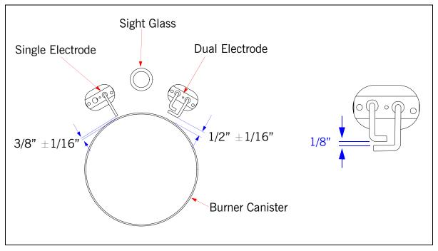
Figure 5-10 Electrode spacing
