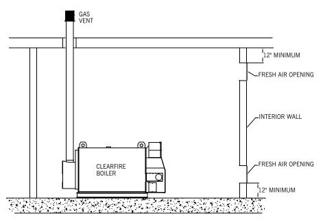
Figure 3-5. Inside Air - Two Opening Method
