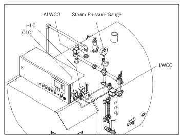
Figure 1-10 CFH Low Water and Limit Controls
