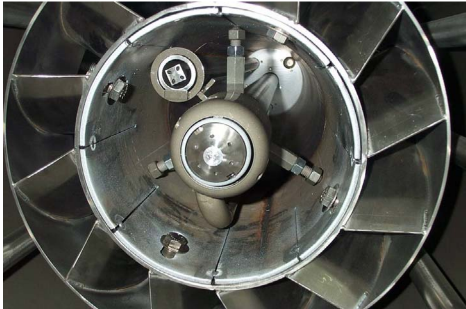
Fig 2: (Addendum) Close-up view of Cleaver-Brooks' Natcom burner showing unique Center Core stabilizing gas injector, which is used to achieve high turndown while maintaining the boiler in hot standby.
