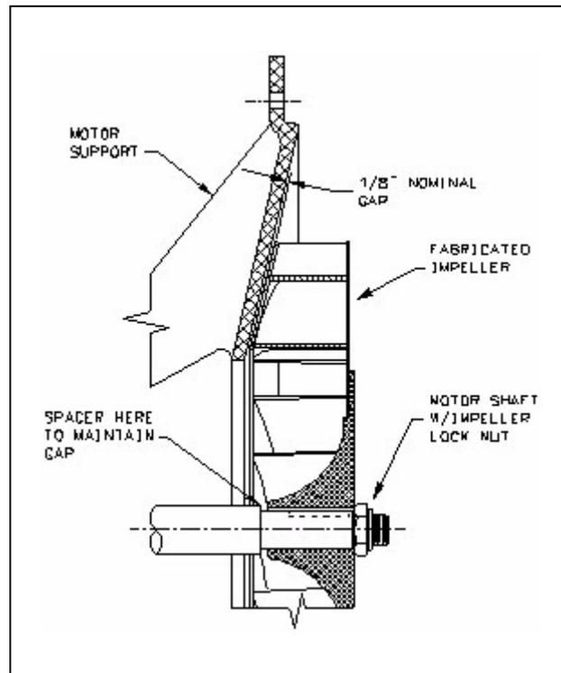
Figure 6-1 Impeller Cutaway
