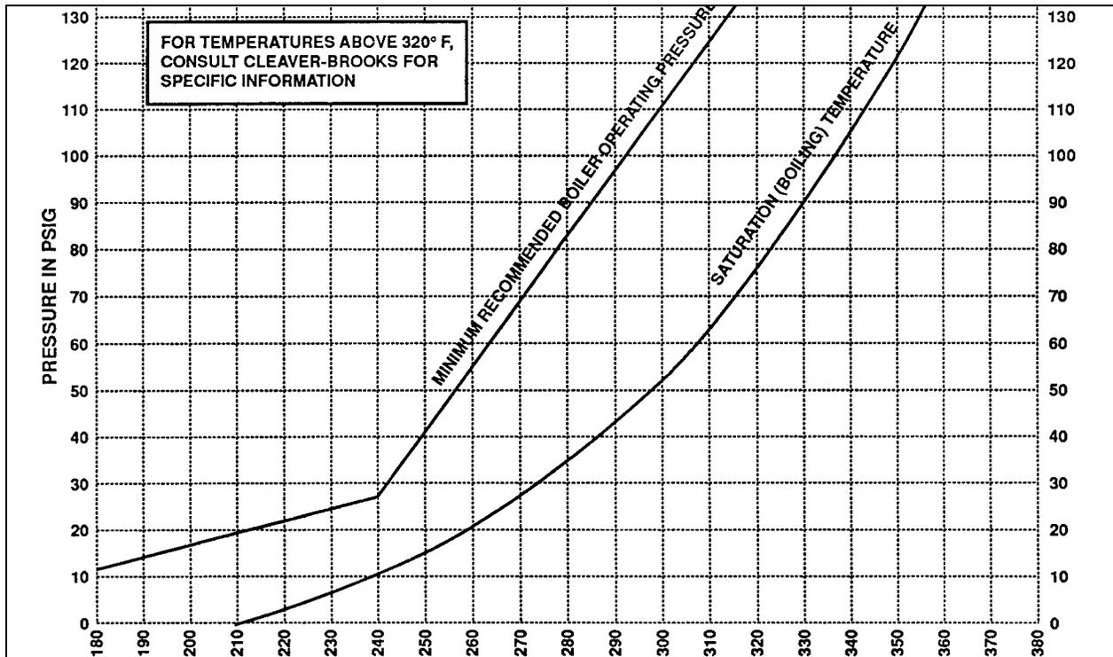
**Figure 2-4. Internal Boiler Pressure**
