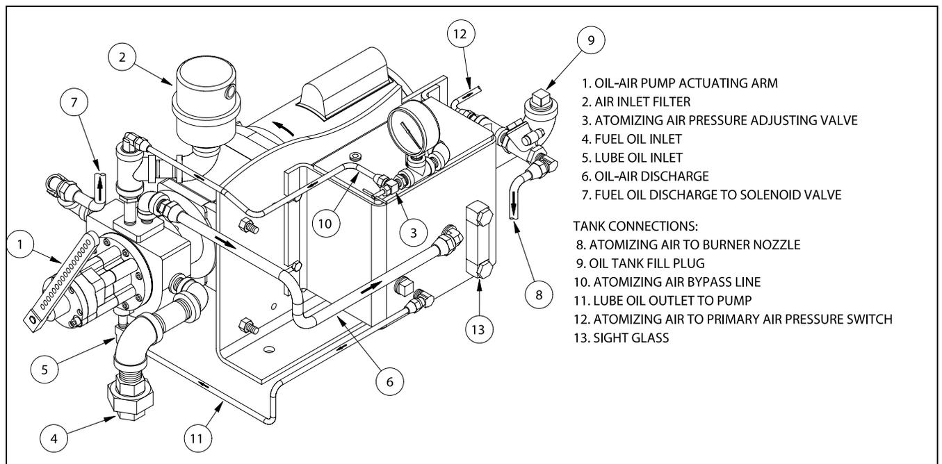
Figure 5-15 Oil Metering Pump and Tank Assembly, Integral Compressor
