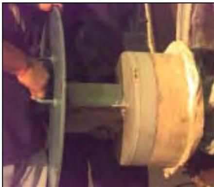
**Figure 2-15 Replacement Of Rear Access Plug**
