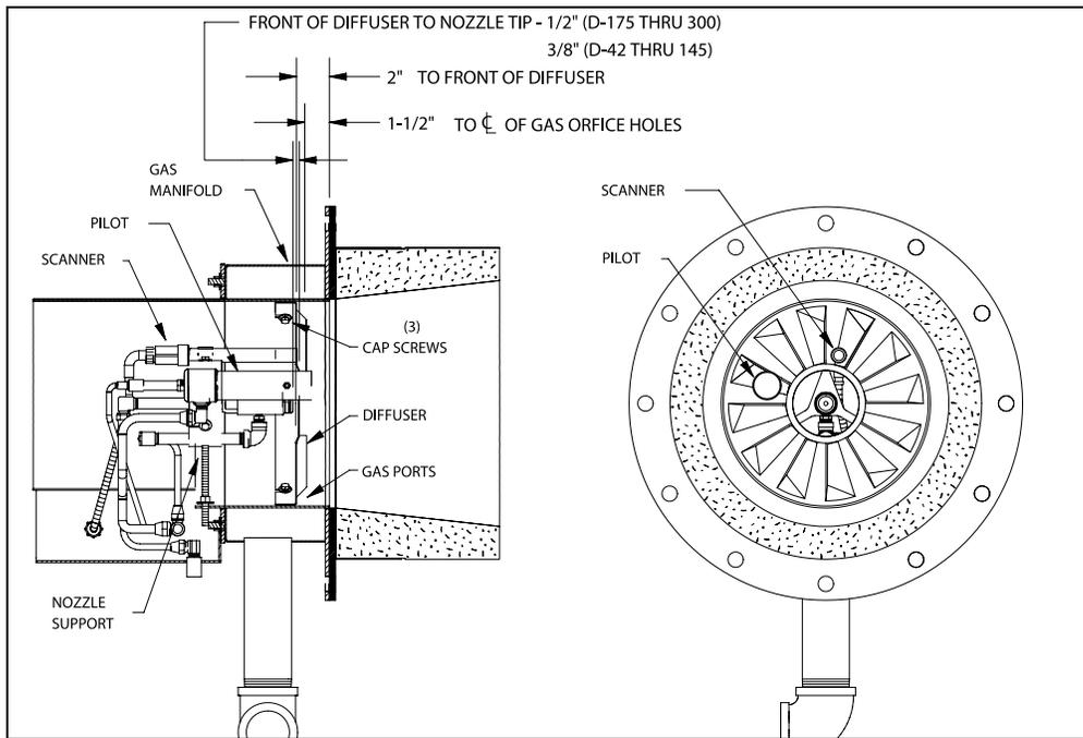
**Figure 6-5 Firing Head Assembly**
