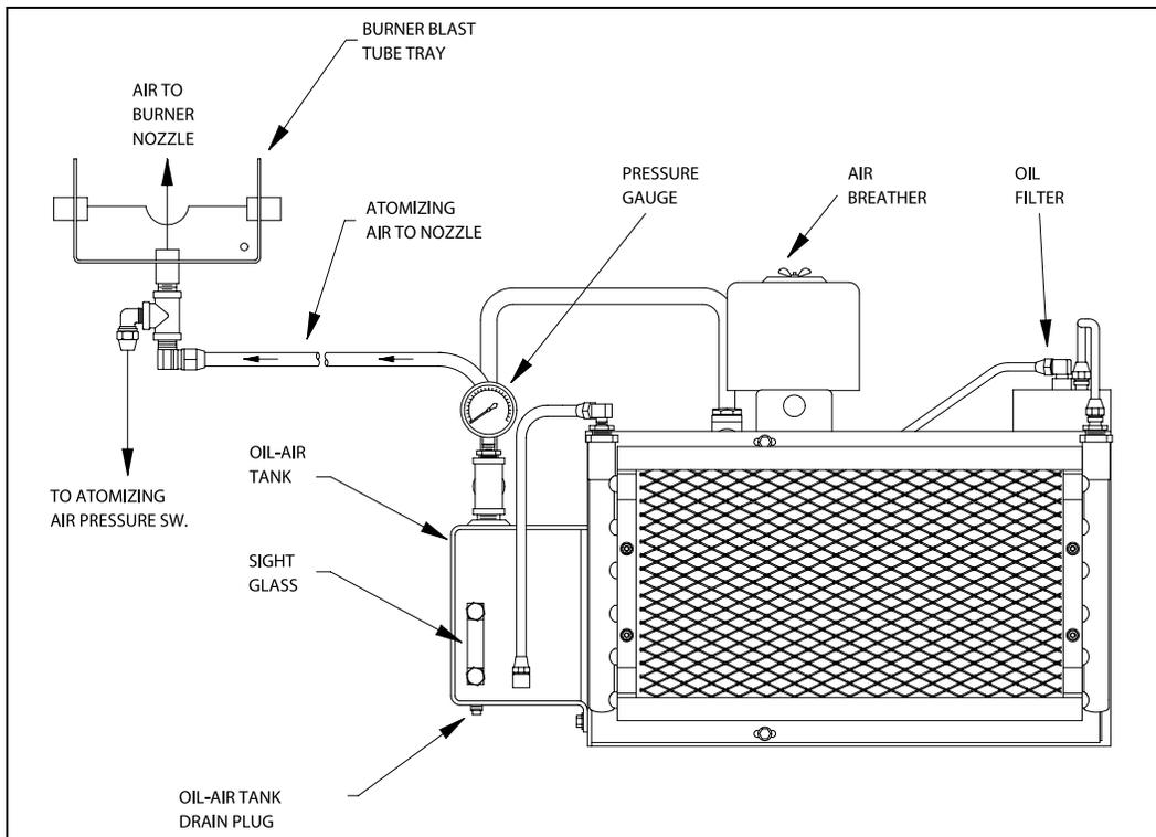
Figure 5-19 Separate Compressor Module
