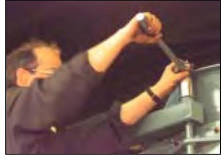
**Figure 2-12 Tighten Davit Nut**
