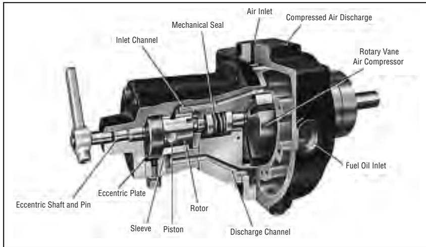
**Figure 5-14 Air Compressor Cutaway**
