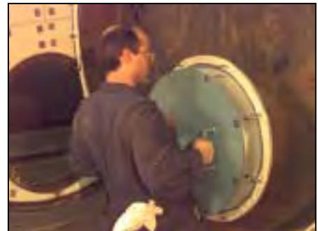
**Figure 2-13 Removing Rear Access Plug**
