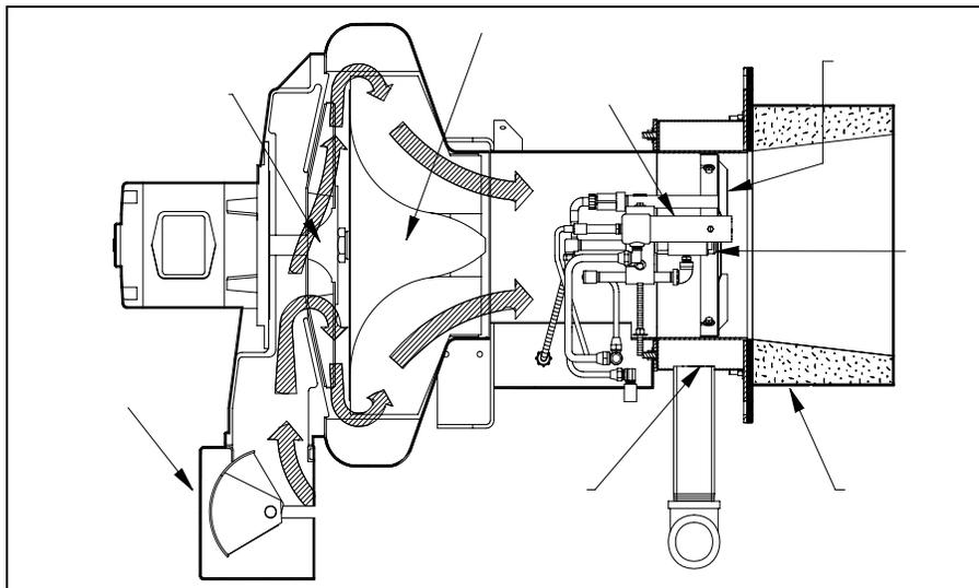
Figure 5-4 Combustion Air Handling System
