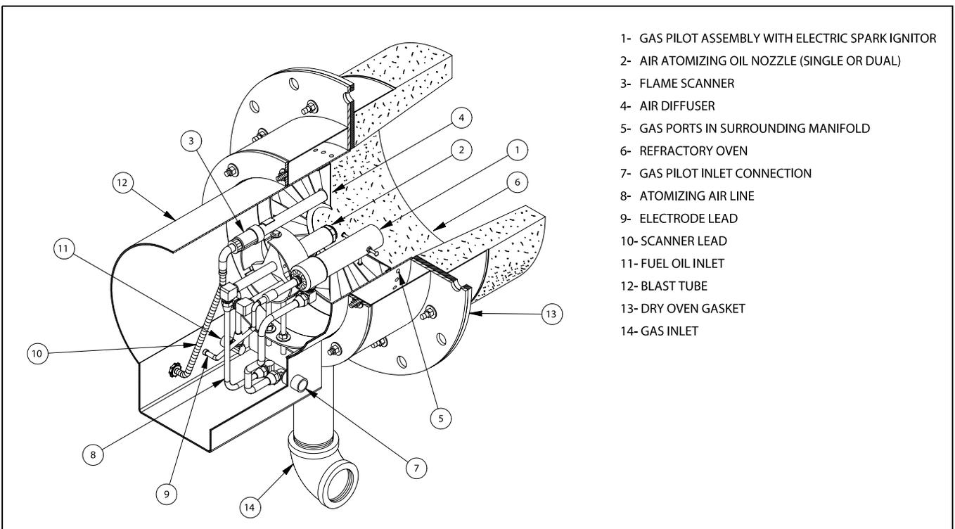
Figure 5-8 Firing Head Assembly
