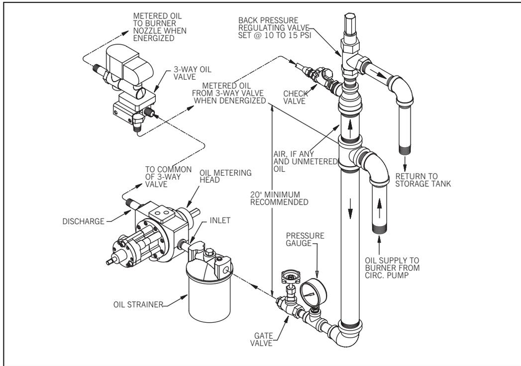
Figure 5-18 Typical Oil Supply Loop
