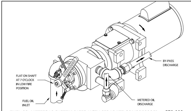
Figure 5-16 Separate Fuel Oil Metering Pump
