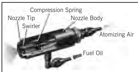
**Figure 6-3 Oil Nozzle Cutaway**
