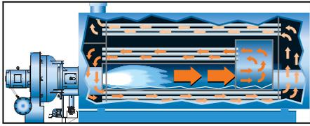
**Figure 1-1 Criterion Boiler Cutaway, Wet-Back Design**
