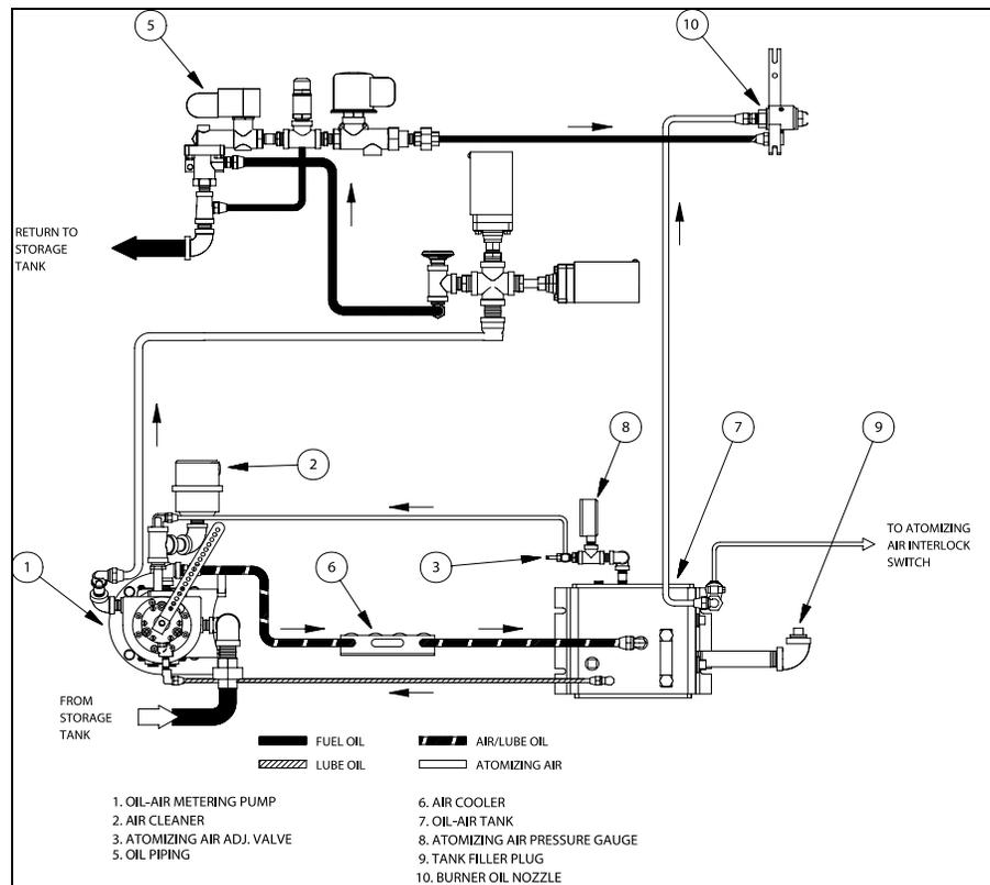
**Figure 5-13 Integral Compressor Oil-Air Metering System**
