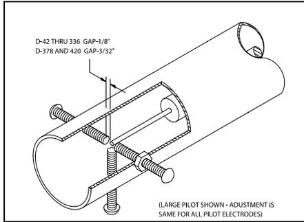
**Figure 6-2 Gas Pilot Electrode**
