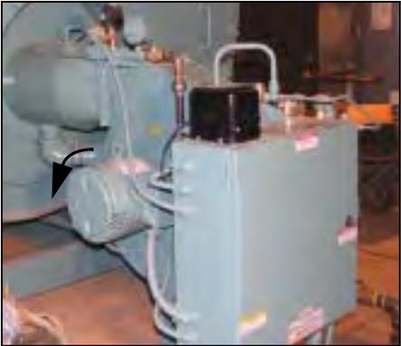
**Figure 4-1 Motor and Fan Rotation**
