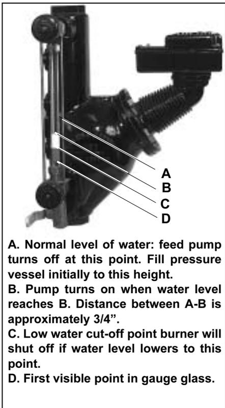
**Figure 2-3. Water Level Gauge Glass**
