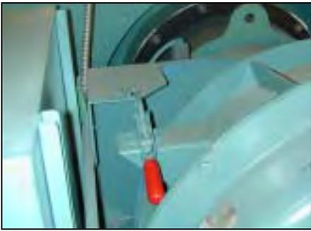
Figure 5-10 Housing Swing Latch
