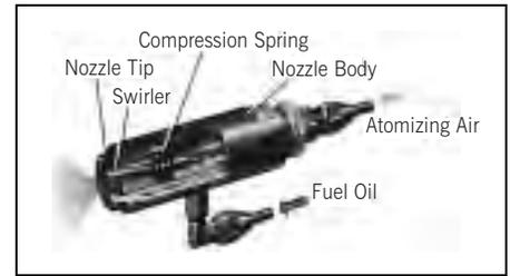
**Figure 5-12 Oil Nozzle Cutaway**
