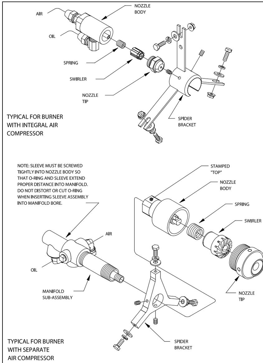
**Figure 6-4 Oil Nozzle Assemblies**
