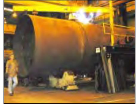
**Figure 1-8 ASME Welding on a Firetube Pressure Vessel**
