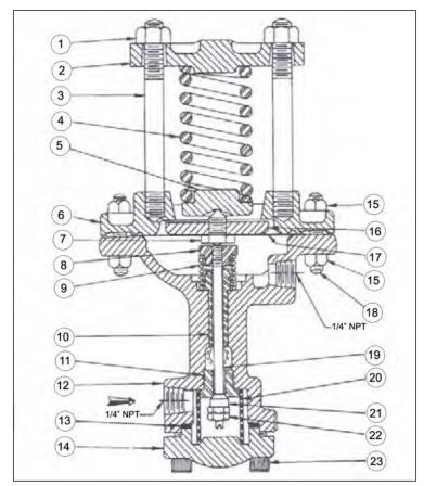
Figure 3-3 Type D Pressure Reducing Cross Section
