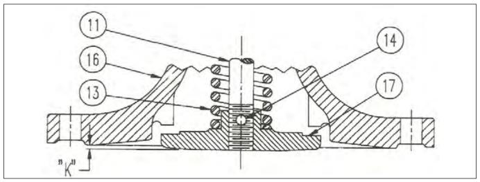
Figure 2-8 Diaphragm Stem Cross Section
