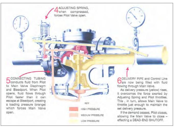
Figure 2-4 The Operating Cycle of a Spence Pressure Regulator
