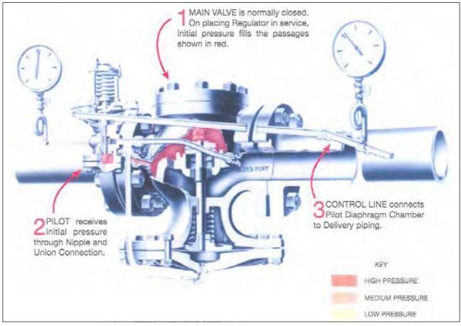
Figure 2-3 The Operating Cycle of a Spence Pressure Regulator
