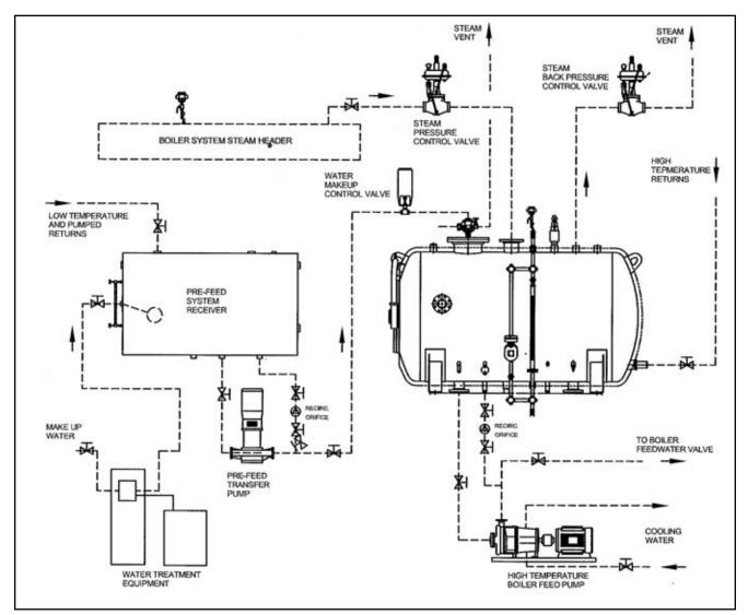
Figure A-2 High Pressure Deaerator Flow Schematic
