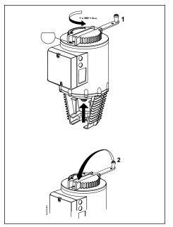
Figure 4-12 SKB/C Automatic Operation
