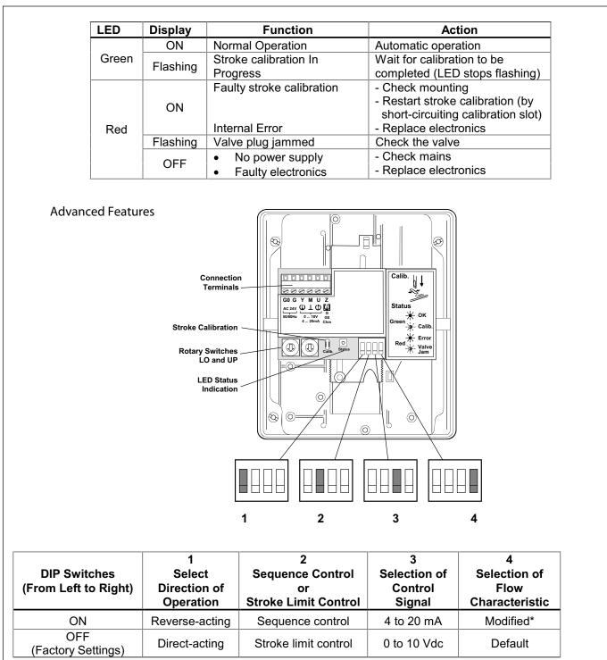
\*Changing the default setting will modify an equal percentage valve to a linear flow characteristic. When set to default, the flow characteristic is determined by the valve body.
