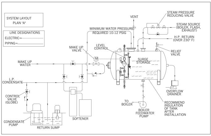
Figure 1-7 System Layout - Plan A
