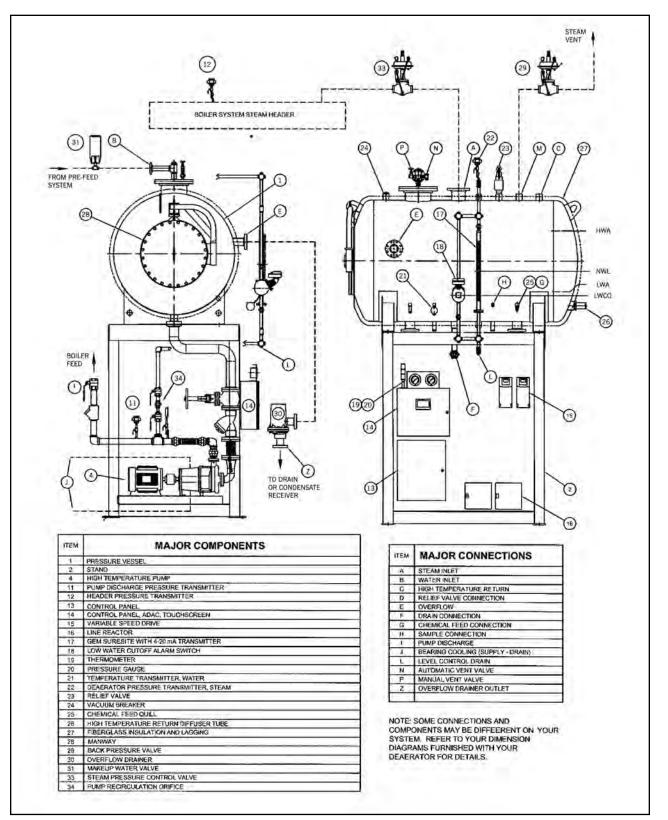
Figure A-1 High Pressure Deaerator Components and Connections
