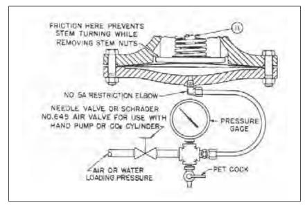
Figure 2-7 Diaphragm Cross Section
