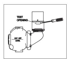
Control can be tested on a deaerator by gently inserting a screwdriver or similar tool in the test opening below the switch (see drawing) and lifting linkage to cause float to drop, thereby simulating a low water condition.
