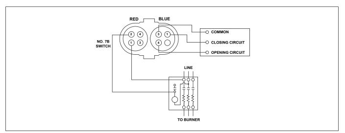
Figure 1-36 Proportional Control, Low Water Cut-Off and Alarm
