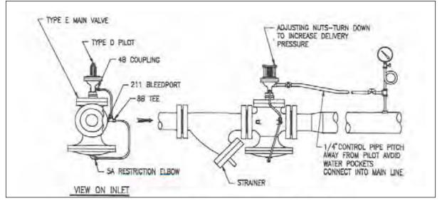
Figure 2-5 Installation of Integrally Mounted Pilot
