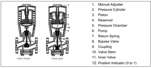
Figure 4-2 SKB/C Valve Parts
