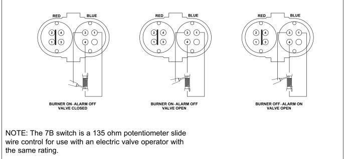
Figure 1-35 Series 93/193 or 94/194 with 7B or 7B-M
