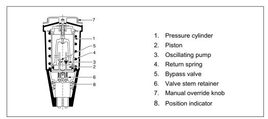
Figure 4-3 SKD Valve Parts
