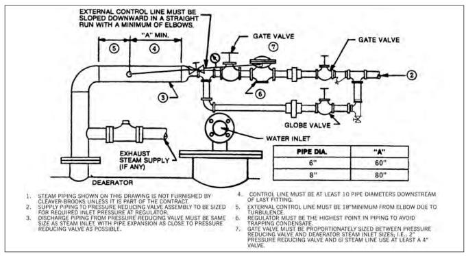
Figure 1-9 Steam Piping for Spraymaster Deaerators
