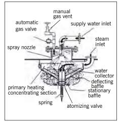
Figure 1-5 Spray Head Components
