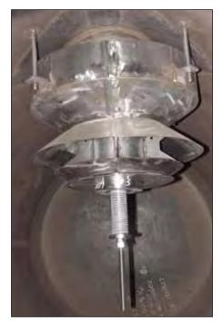
Figure 1-6 Spray Head Installed
