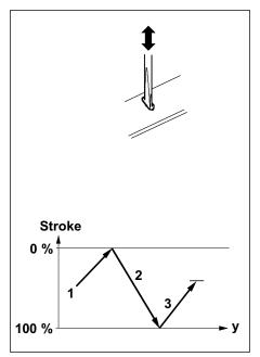
Figure 4-7 Automatic Calibration
