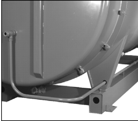
Figure 8-24 Rear Door with Site Glass Cooling Tube
