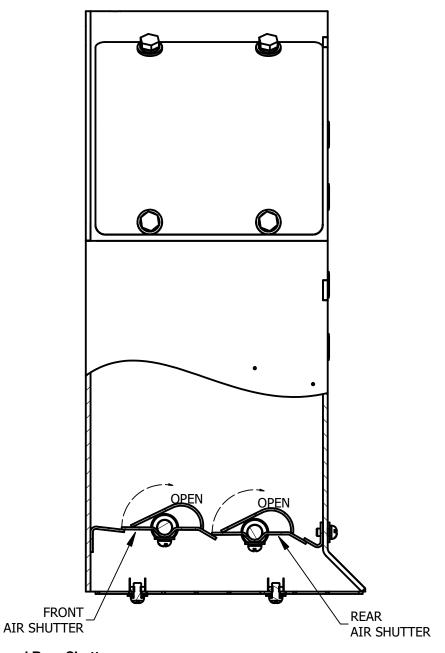
FIGURE 4-26. Front and Rear Shutters
