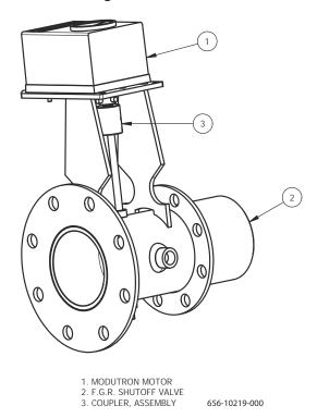
FIGURE 7-3. FGR Shutoff Valve
