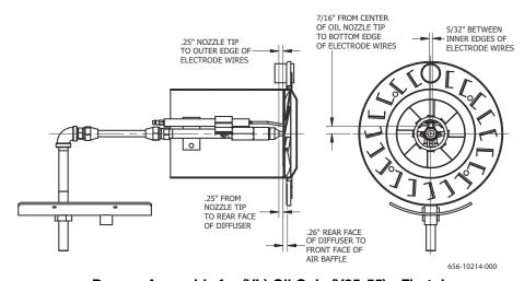
FIGURE 4-7. Drawer Assembly for (VL) Oil Only (V35-55) - Firetube
