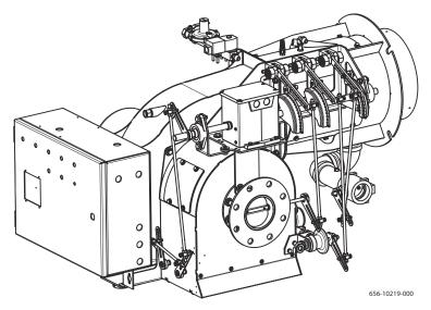
FIGURE 7-1. General Layout of the Burner
