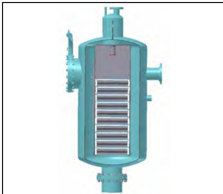
Figure 1-2 Tray column - section view
