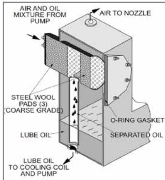
FIGURE 8-17. Air-Oil Receiver Tank
