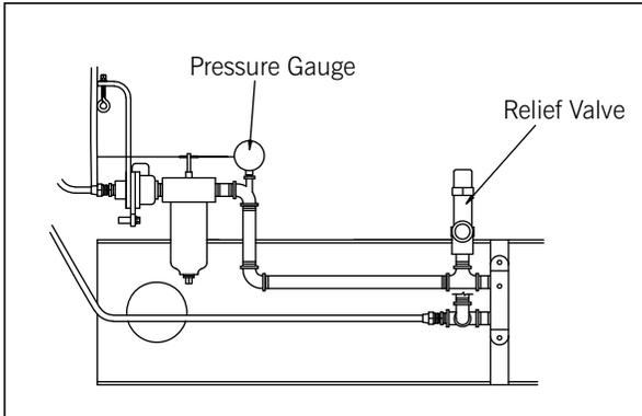
Oil supply pressure is regulated by adjusting the pressure relief valve at the oil terminal block. A pressure gauge should be installed in the terminal block and the relief valve adjusted to obtain a minimum reading of 75 psi when the burner is firing at maximum rate.
