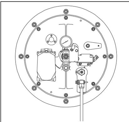
**FIGURE 5-3. Burner Drawer with Damper Actuator**
