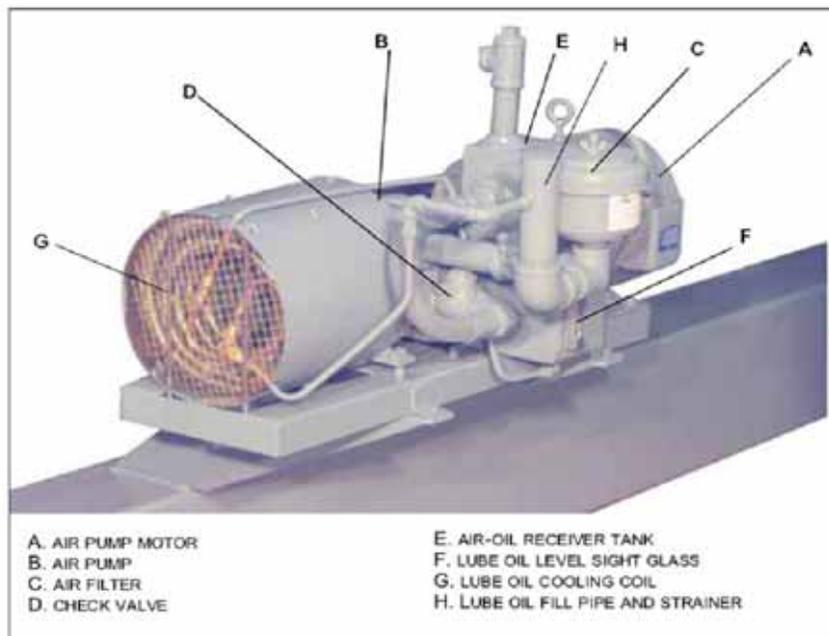
FIGURE 2-4. Air Pump (Primary Air)
