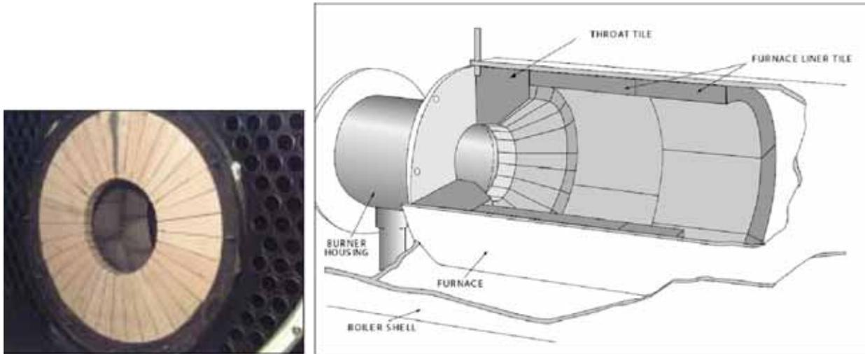
**FIGURE 8-19. Throat Tile and Furnace Liner**
