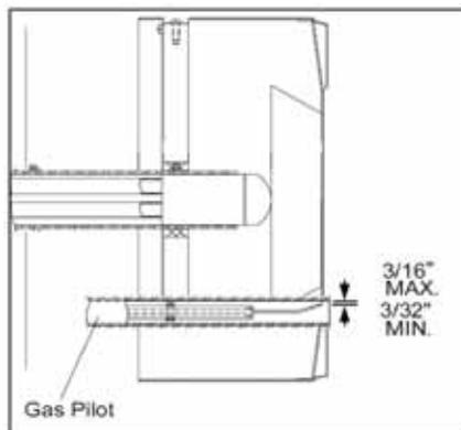
**FIGURE 6-8. Gas Pilot Electrode**
