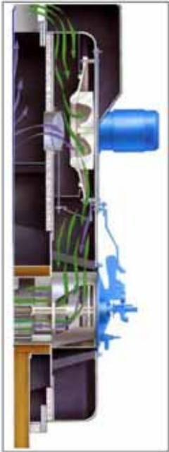
The low emission option for the CBEX Elite line of Firetube Boilers reduces Nitrogen Oxide (NO<sub>x</sub>) emissions, a major contributor to ozone pollution (smog). Carbon Monoxide (CO) emissions also tend to be lower as increased turbulence caused by the addition of the flue gases into the combustion air stream results in improved combustion.
