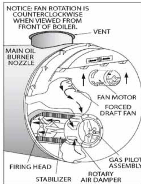
FIGURE 2-5. Secondary Air Flow Diagram
