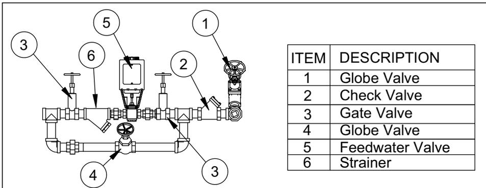
FIGURE 3-4. Feed piping, typical
