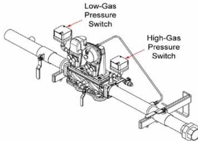
**FIGURE 6-6. Gas Train Pressure Switches**
