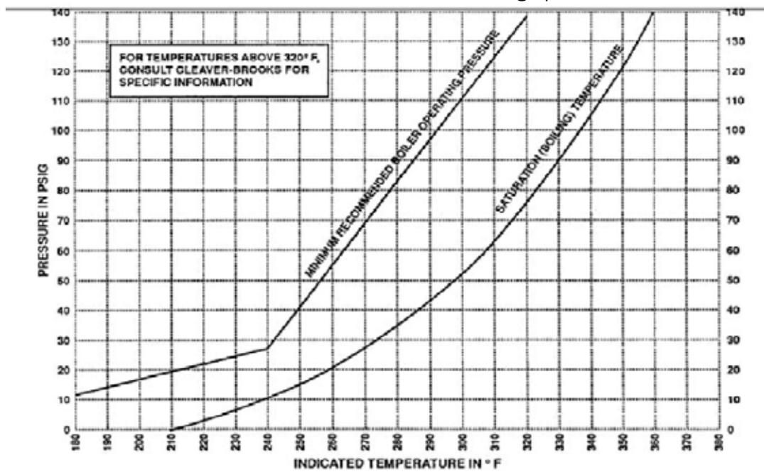
**FIGURE 3-3. Internal Boiler Pressure**
