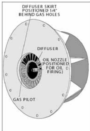
There are relatively few adjustments that can be made to the burner, however, a check should be made to assure that all components are properly located, and that all holding screws are properly tightened.
