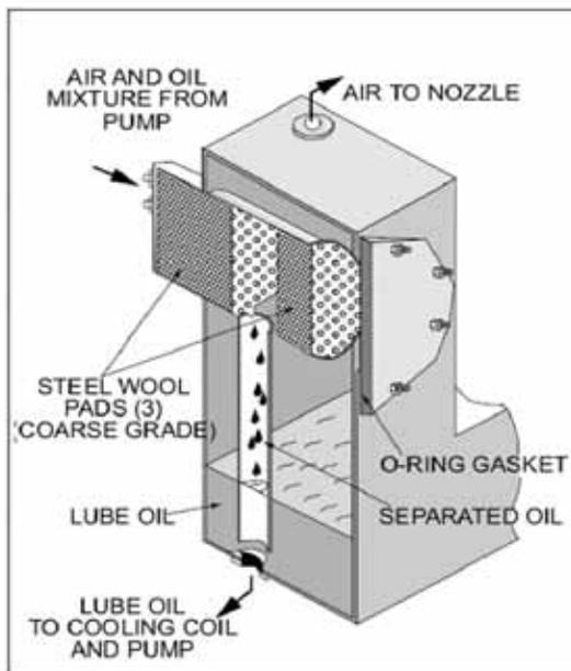
FIGURE 2-6. Air-Oil Receiver Tank
