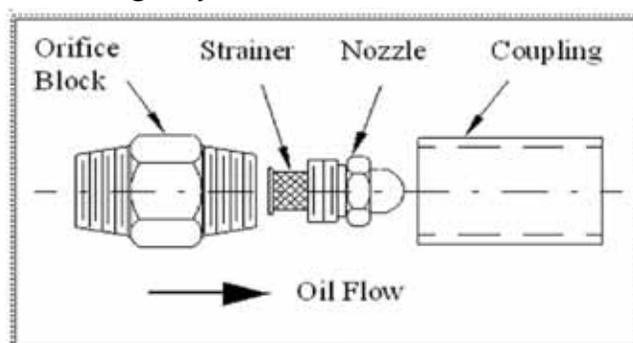
**FIGURE 8-8. Back Pressure Orifice**
