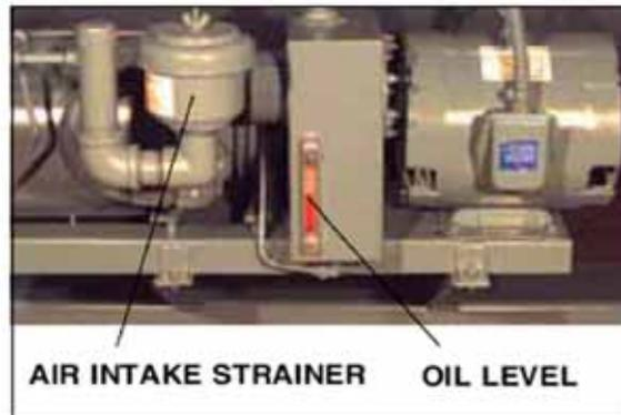
**FIGURE 5-2. Atomizing Air Pump**
