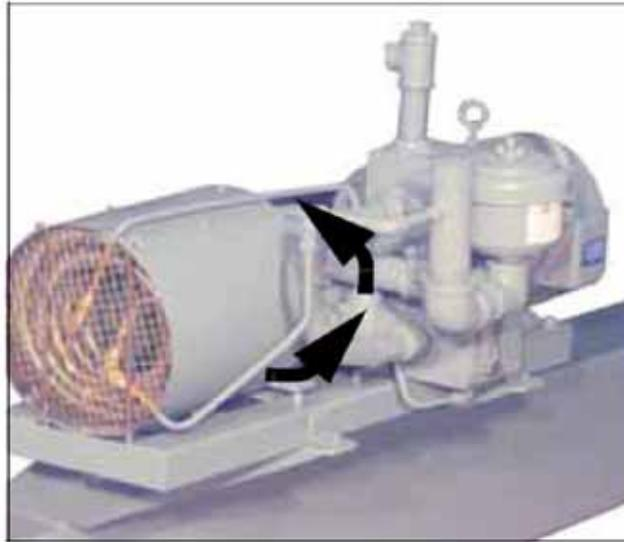
**FIGURE 5-1. Air Compressor Motor Rotation**
