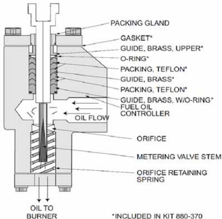
FIGURE 8-15. Fuel Stem Packing, Cross-Section
