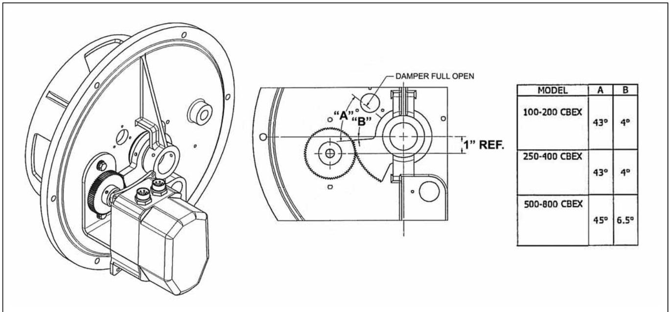
FIGURE 8-10. Rotary Air Damper
