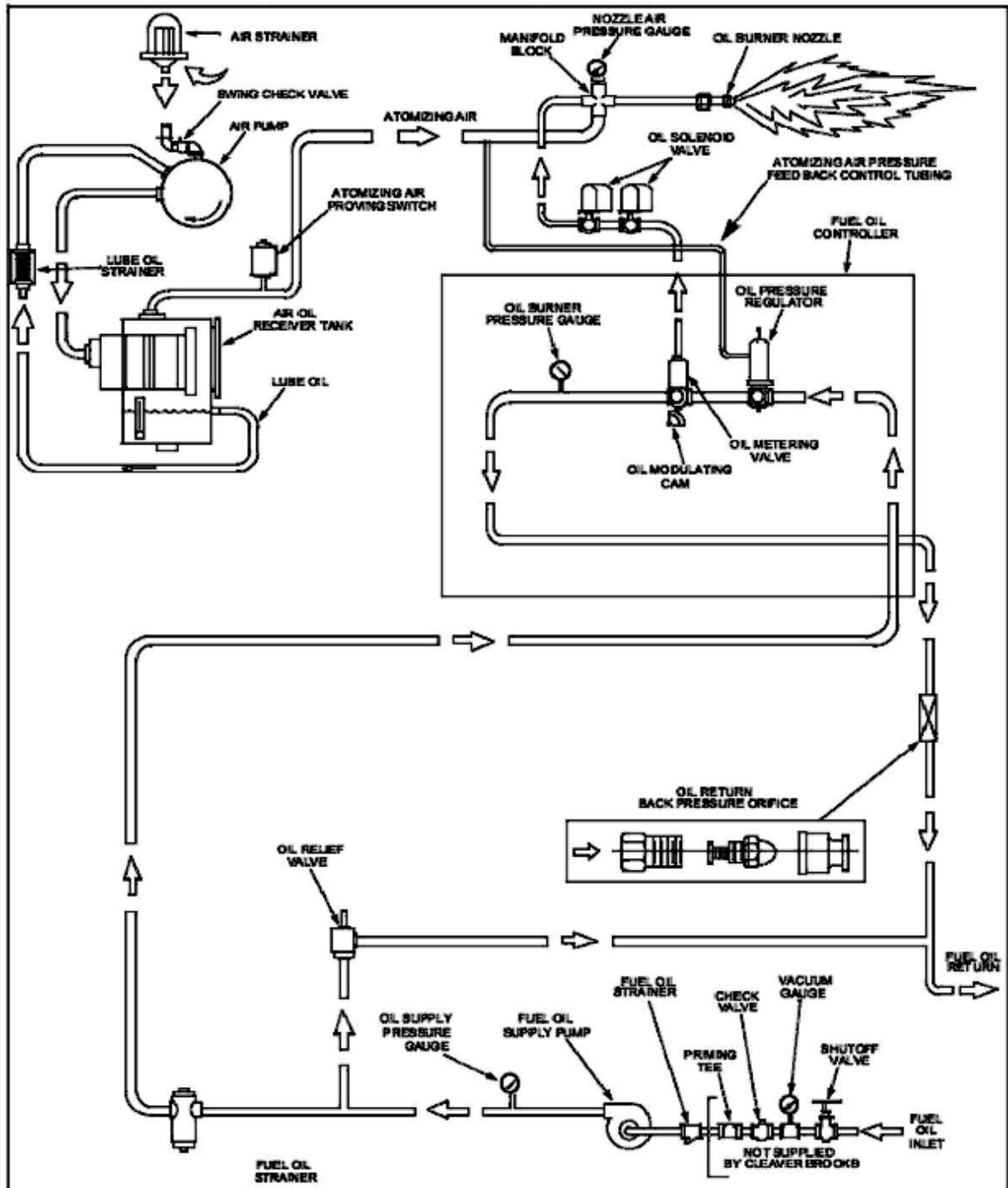
FIGURE 2-7. Diagram for Light Oil Flow
