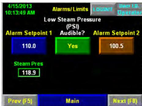
Figure 5-22. Alarms and Limits - Low Steam Pressure
