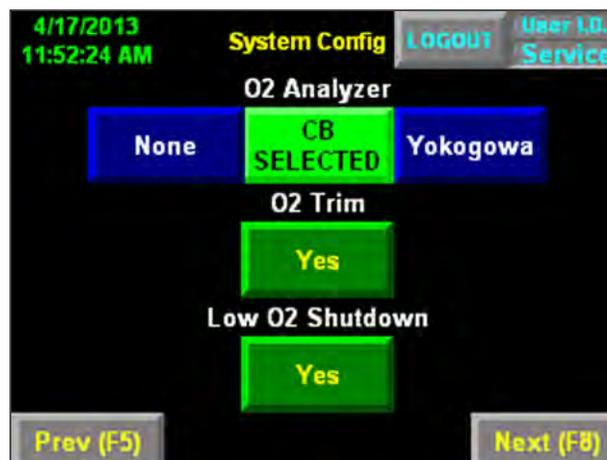
Figure 4-18. O<sub>2</sub> Analyzer
