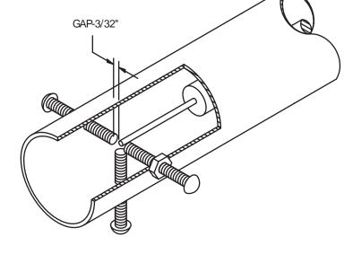
Figure 3-11: Ignition Pilot Electrode Setting
