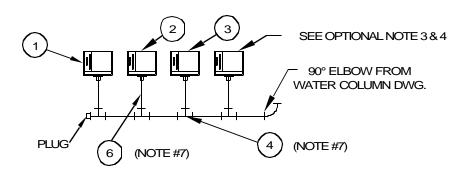
PRESSURE SWITCH PIPING FOR 15-300 PSI CBL
