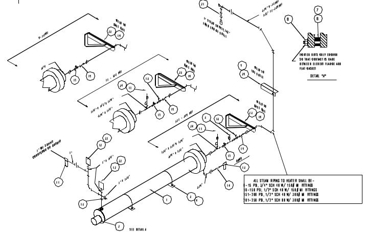
INSTALL., ST/ELEC. HTR & PIPING #6 OIL,CBL,0-250PSI,200-600V
