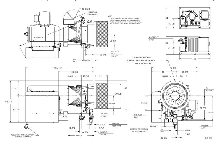
Figure 3-4: Burner Dimensions
