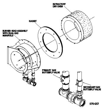
Figure 3-1: Firing Head Assembly
