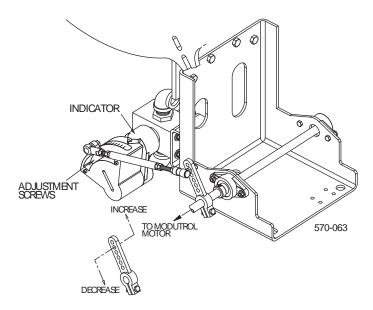
Figure 3-8: Cam Linkage
