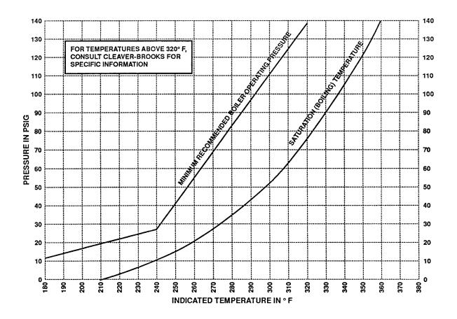
Figure 2-2: Internal Boiler Pressure
