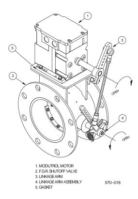
Figure 3-15: Mod Motor Orientation
