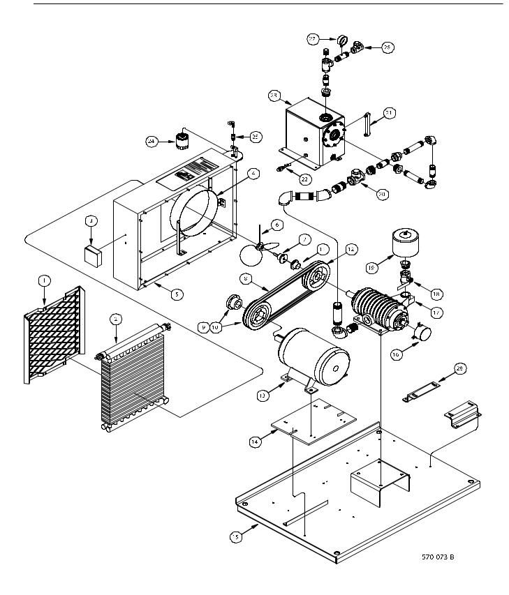
Figure 6-14: Separate Compressor Assembly
