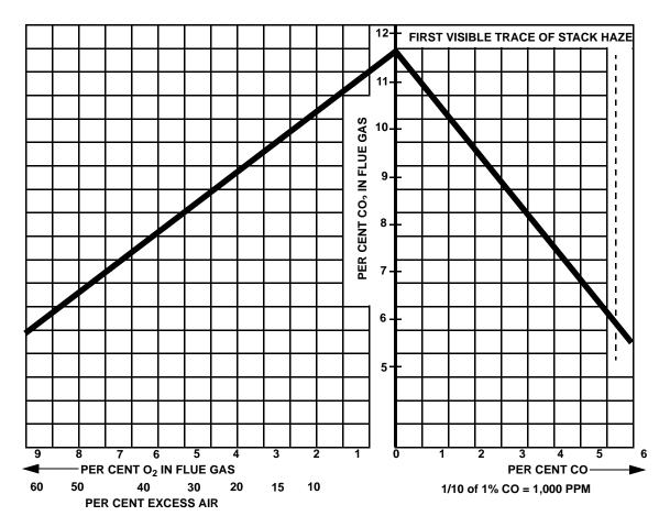
Figure 4-6: Flue Gas Analysis Chart for Natural Gas
