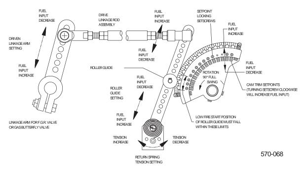
Figure 3-7: Fuel Cam and Linkage Components
