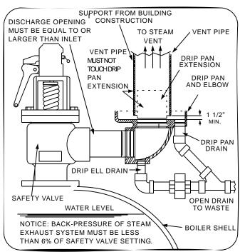
Figure 1-7: Recommended Piping For Steam
