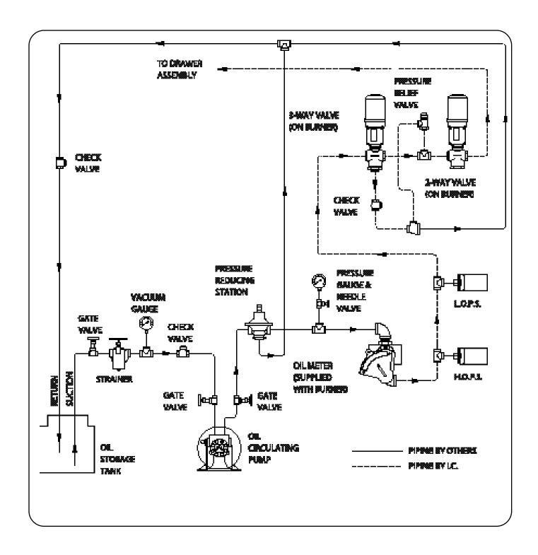
Figure 3-2: Oil Piping Arrangement
