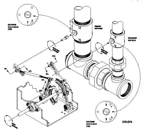
Figure 3-6: Butterfly shaft slot indicated valve angle
