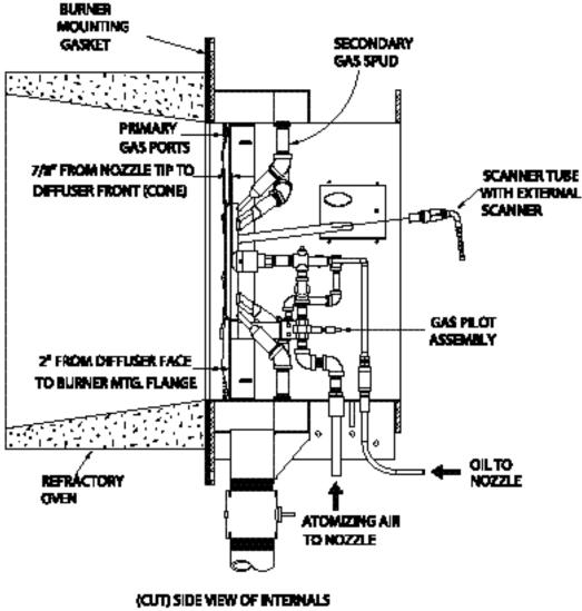
(CUT) SIDE VIEW OF INTERNALS. FIRING HEAD ASSEMBLY
