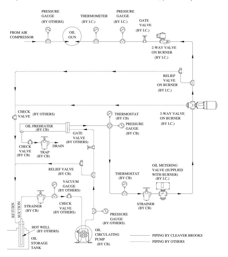
Figure 3-17: Schematic Diagram For No. 6 Heavy Oil Flow (W/S1 BURNER) (STEAM-ELECTRIC HEATER)
