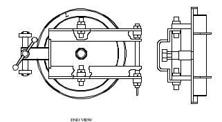
Sealing the rear access plug requires cleaning the seal area. Spray adhesive into the sealing area and insert the 2" rope gasket.
