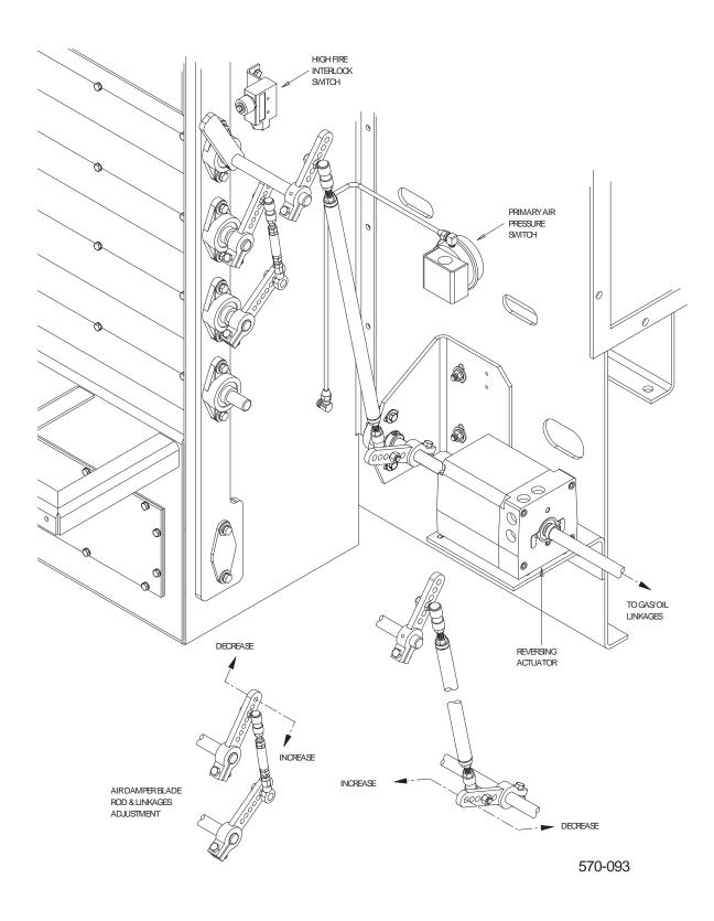
Figure 3-9: Air Damper Linkage
