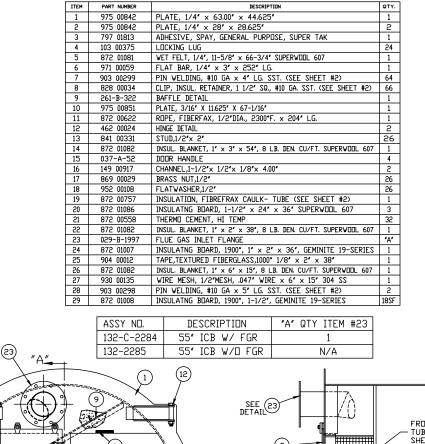
Figure 10-7. Smoke Box 55" 100-125 HP 4 Pass
