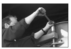
Figure 9-10. Tighten Davit Nut
