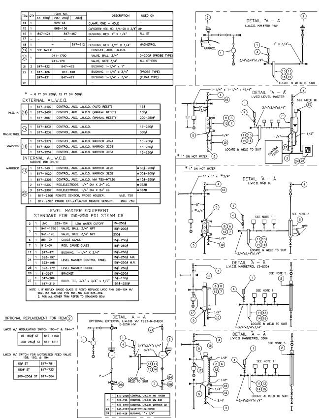
Figure 10-18. Water Column Piping 100-200HP (55" & 60")
