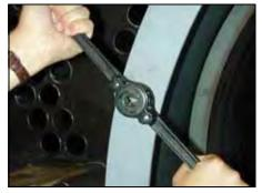
Figure 9-11. Use Thread Die to Chase Threads if Damaged
