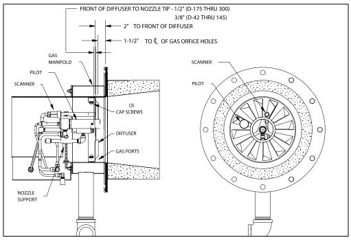
Figure 7-5. Firing Head Assembly
