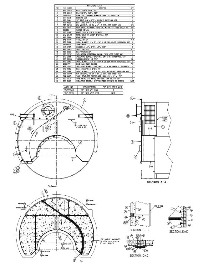
Figure 10-11. Smoke Box 92" 500-600 HP 4 Pass
