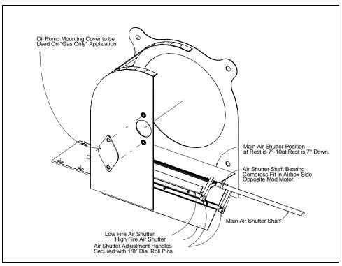
Figure 4-10. Air Box and Air Shutters
