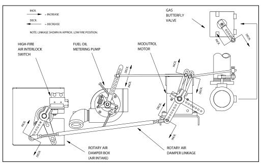
Figure 7-6. Firing Rate Controls
