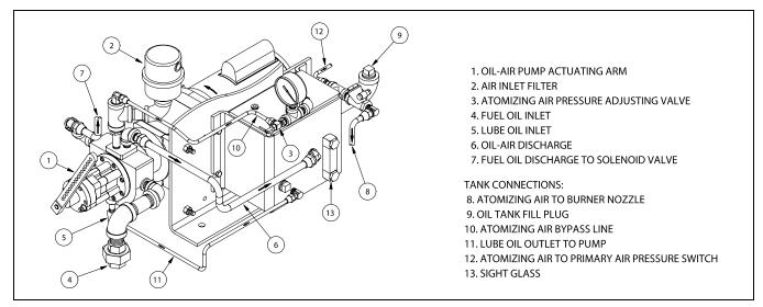
Figure 6-13. Oil Metering Pump and Tank Assembly, Integral Compressor
