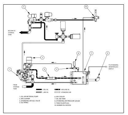
Figure 6-11. Integral Compressor Oil-Air Metering System
