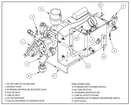
Figure 7-7. Integral Oil Air Metering System and Tank
