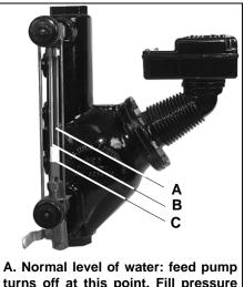
A. Normal level of water: feed pump turns off at this point. Fill pressure vessel initially to this height.
