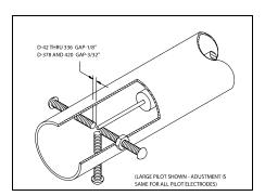
Figure 7-2. Gas Pilot Electrode
