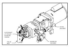
Figure 6-14. Separate Fuel Oil Metering Pump
