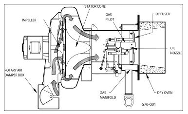
Figure 6-4. Combustion Air Handling System
