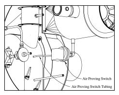
Figure 5-7. Combustion Air Proving Switch
