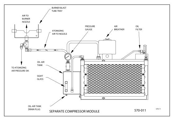
Figure 6-17. Separate Compressor Module
