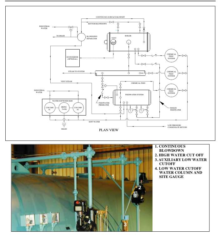
Figure 2-4. Low-Water Cutoff Auxiliary Low Water Cutoff and High Water Cutoff
