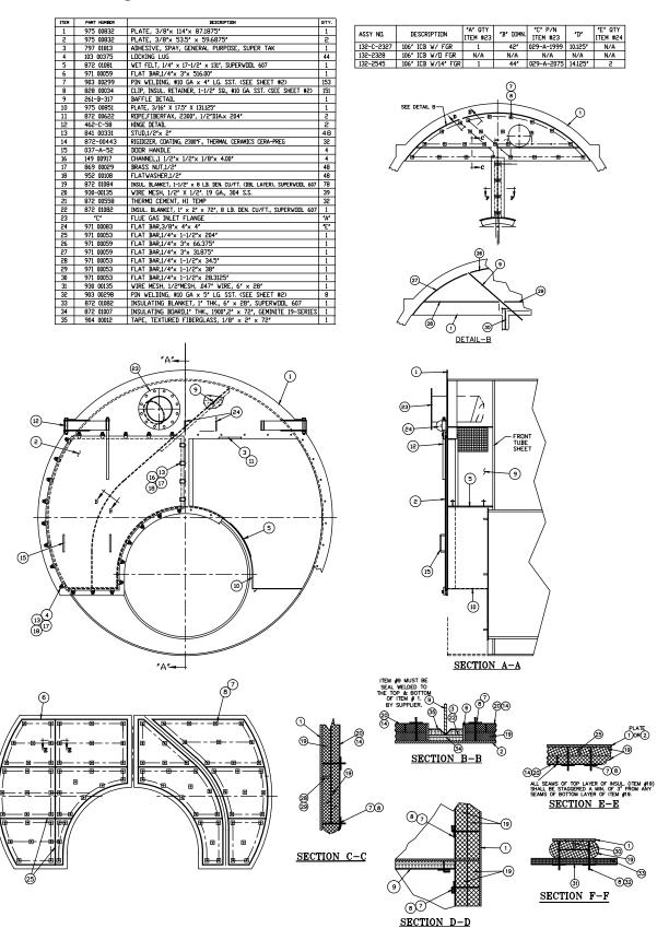
Figure 10-12. Smoke Box 106" 700-800 HP 4 Pass
