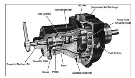
Figure 6-12. Air Compressor Cutaway
