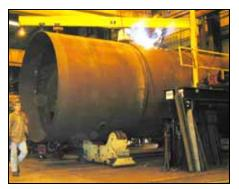
Figure 1-7. ASME Welding on Firetube Boiler
