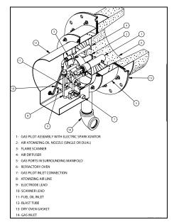
Figure 9-7. Burner Head "D" Series
