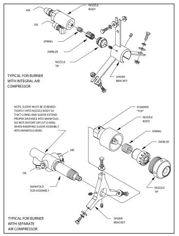
Figure 7-4. Oil Nozzle Assemblies
