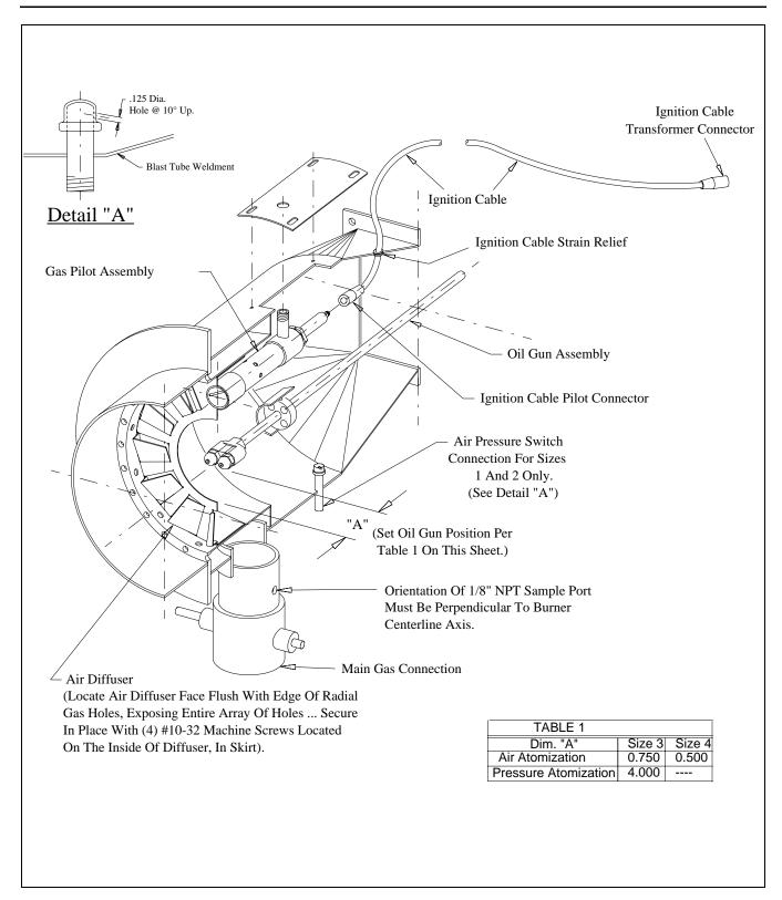
Figure 4-12. Blast Tube and Diffuser Start-Up Dimensions
