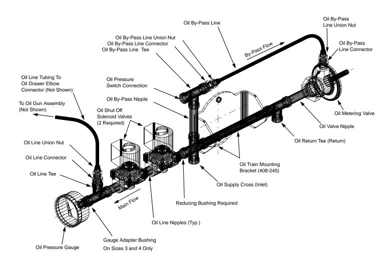
Figure 10-12. Remote Pump, Pressure Atomized Light Oil (Opt. Oil, Gas-Oil Fired Units, 100-150 HP)
