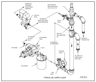
Figure 6-16. Typical Oil Supply Loop
