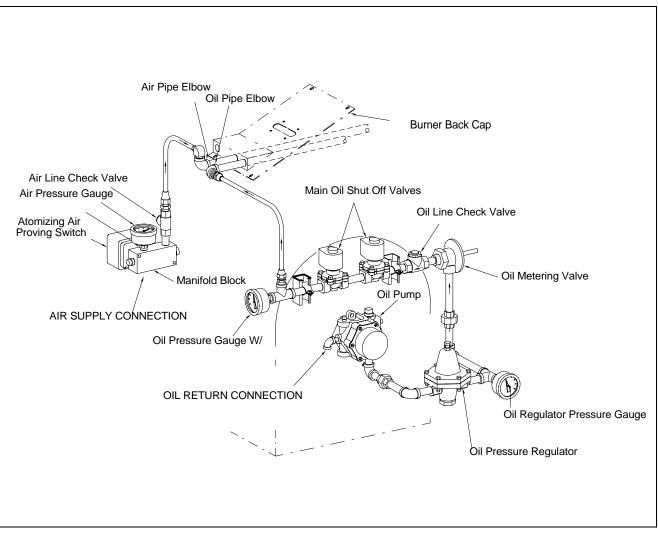
Figure 4-6. ProFire Burner Air Atomized, Direct Drive System (Light Oil)
