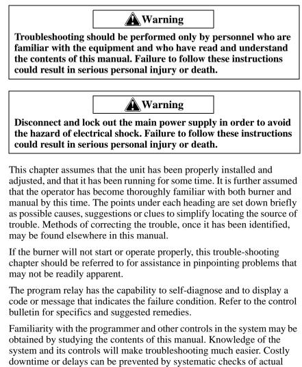
downtime or delays can be prevented by systematic checks of actual operation against the normal sequence to determine the stage at which performance deviates from normal. Following a routine may possibly eliminate overlooking an obvious condition, often one that is relatively simple to correct.
