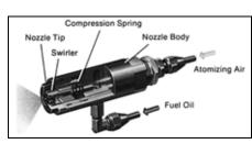
Figure 6-10. Oil Nozzle Cutaway
