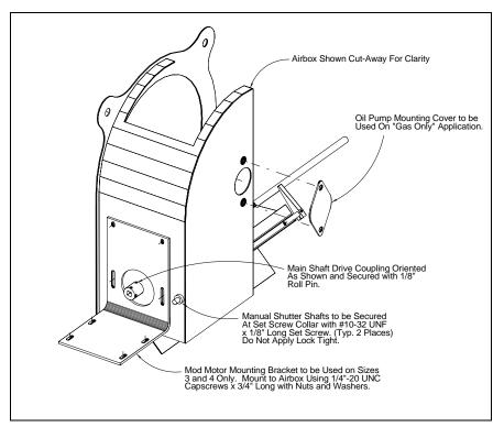
Figure 4-11. Air Box and Air Shutters
