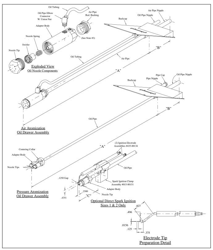
Figure 9-9. "F" Series Burner Nozzle and Electrode
