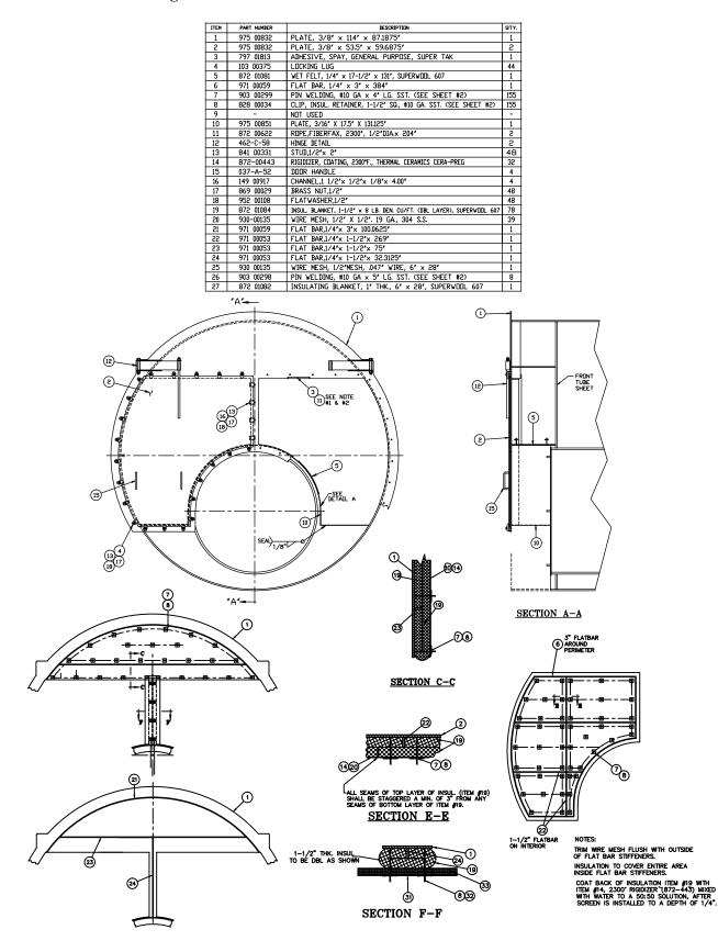
Figure 10-6. Smoke Box 106" 700-800 HP 3 Pass
