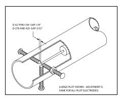
Figure 9-8. Ignition Pilot "D" Series Burner
