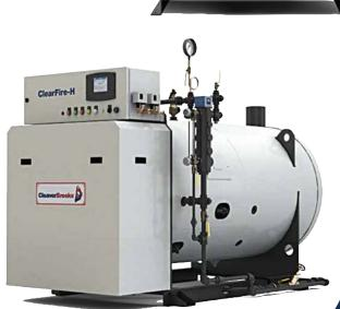
**ClearFire-H** is a traditional horizontal high and low pressure steam boiler design (15# and 150#) with sizes ranging from 10 – 60 HP and 85% efficient (87% with economizer).
