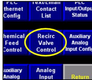
Recirculation valve control is available on single tank applications.
