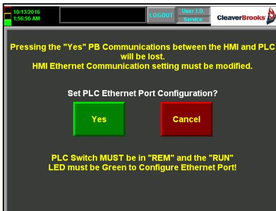
**NOTE:** The PLC must be in REM and the RUN LED must be GREEN to configure the Ethernet port.
