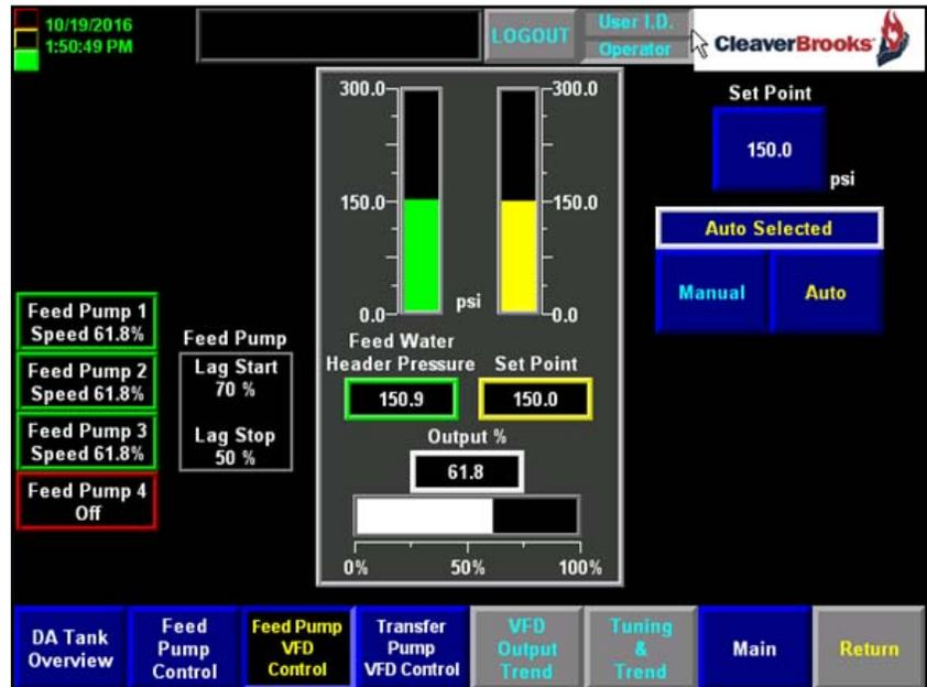
Figure 3-22 Pump VFD Control - Auto
