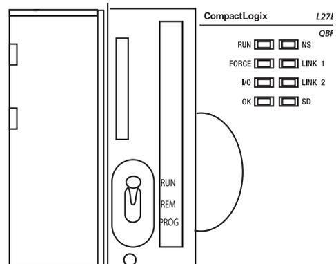
The PLC and associated devices are mounted on a DIN rail in the ADAC control panel.
