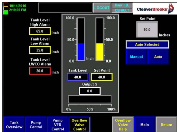
Figure 3-33 Overflow Valve Control
