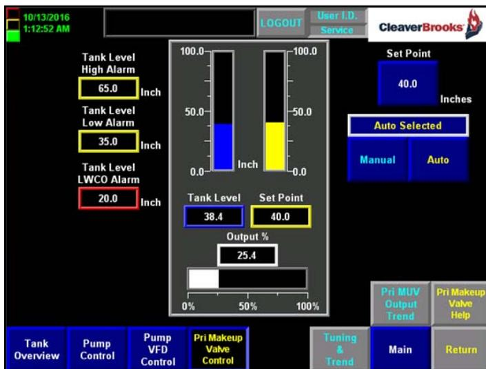
Figure 3-26 Primary Makeup Valve Control
