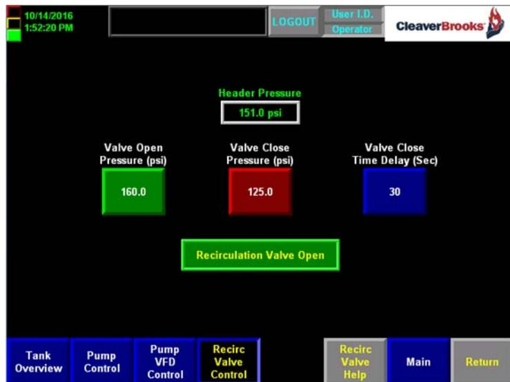
Figure 3-35 Recirculation Valve Control
