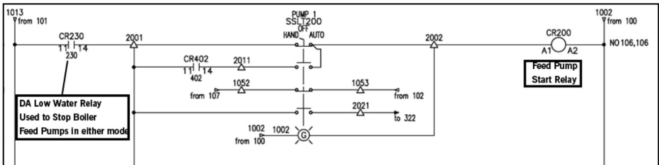
Figure 3-39 DA Bypass Wiring 2 of 2
