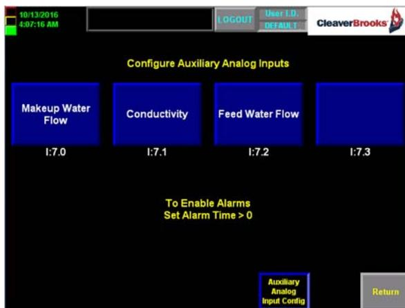
Figure 3-40 Aux analog input single tank
