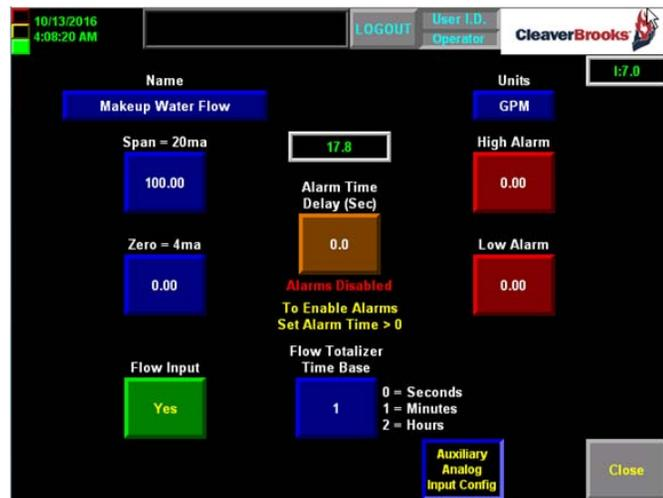
Figure 3-42 Aux analog input configuration (continued)
