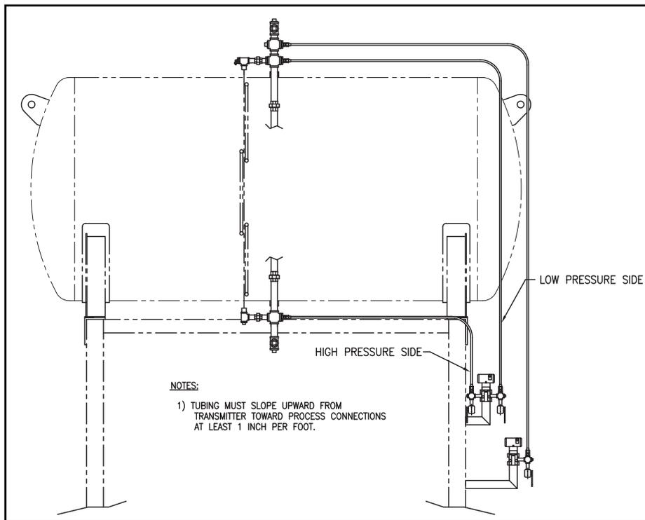
Differential Pressure Level Control and DA Tank Pressure Control (2 of 2)
