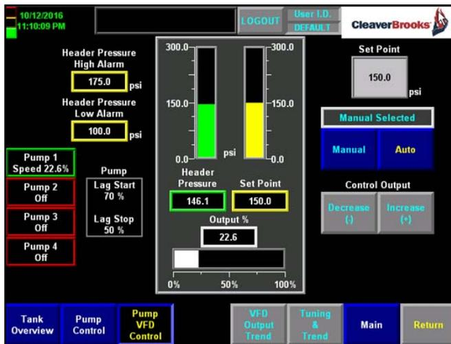
Figure 3-21 Pump VFD Control – Manual
