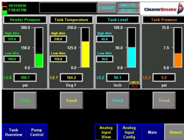
Figure 3-15 Analog Input View - single tank
