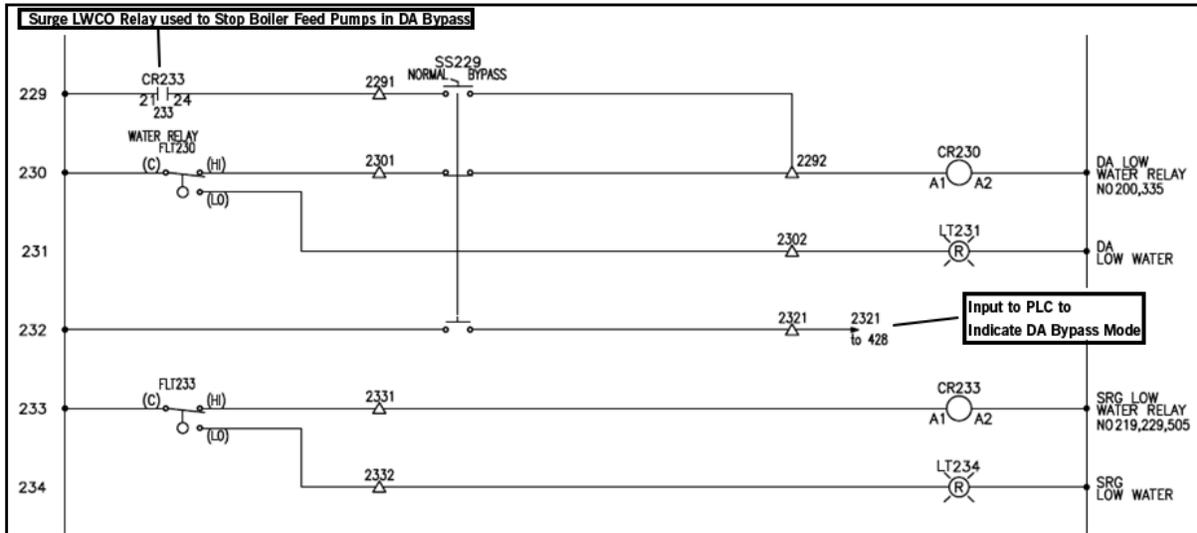
Figure 3-38 DA Bypass Wiring 1 of 2
