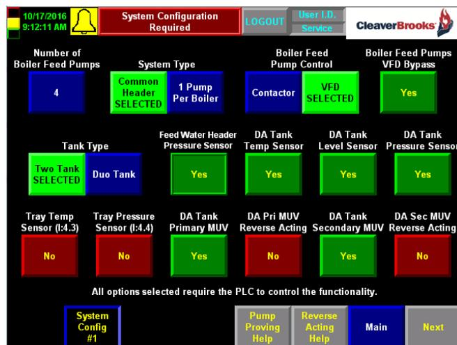
Figure 3-6 System Config 1 - Dual Tank
