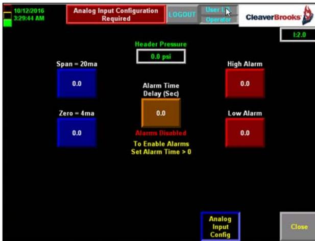
**Figure 3-13 Configure Selected Input (Header Pressure)**
