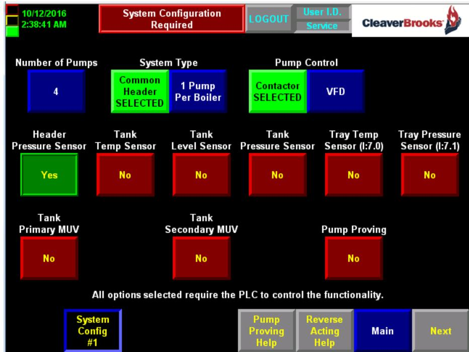
Figure 3-4 System Configuration 1
