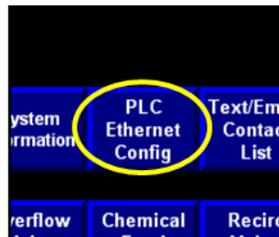
“View Current PLC Ethernet Configuration” shows the current Ethernet settings as read from the PLC.
