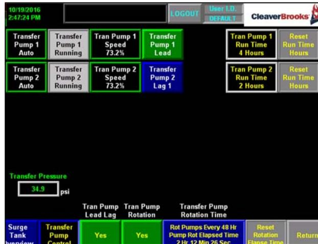
Figure 4-6 Transfer Pump Control Screen
