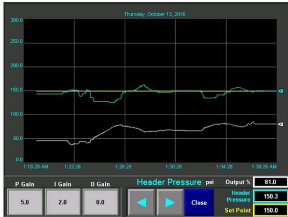
**Figure 3-25 Pump VFD Tune & Trend**
