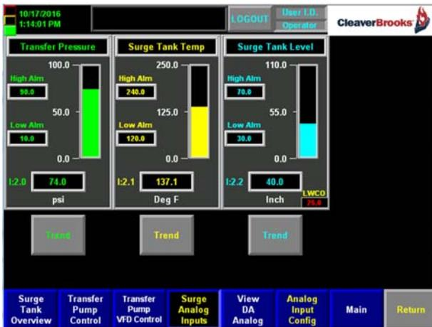
Figure 3-16 Analog Input View - surge tank
