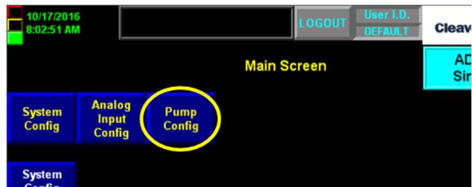
Operator-level login is required to set pump configuration values. No login is required to enable/disable pump functions.
