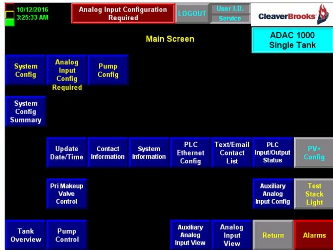
Figure 3-11 System Config complete
