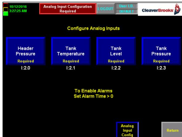
Figure 3-12 Analog Input Configuration select
