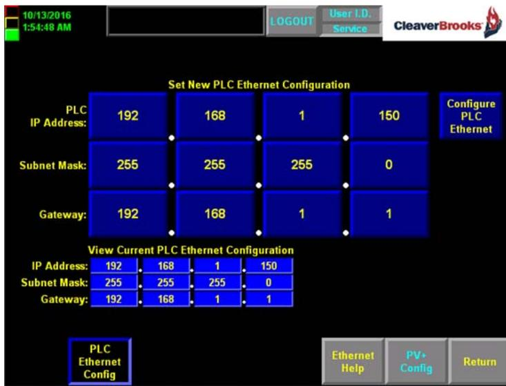
Figure 3-44 PLC Ethernet Configuration
