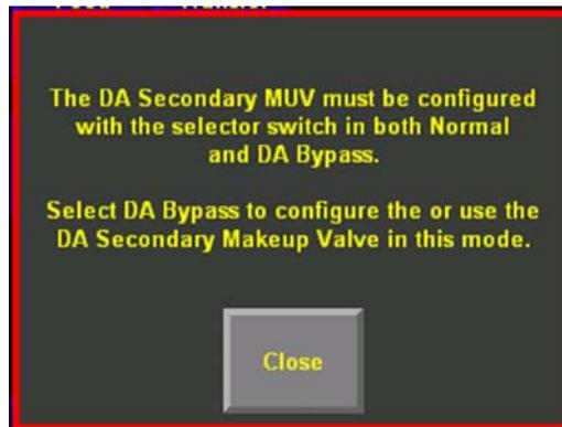
In DA Bypass mode, no matter the makeup valve configuration the DA primary makeup valve control output is snapped to zero and the PID is snapped to manual mode.
