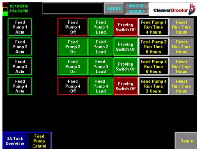
Figure 3-20 One Pump per Boiler
